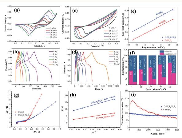
Fig. 4 Electrochemical performance measurements. (a) CV curves of CoNi<sub>2</sub>O<sub>4</sub>, (b) GCD curves of CoNi<sub>2</sub>O<sub>4</sub> samples, (c) CV curves of CoNi<sub>2</sub>S<sub>4</sub>/  $Ni_3S_2$ , (d) GCD curves of  $CoNi_2S_4/Ni_3S_2$ , (e) b values of two kinds of electrode materials, (f) capacitance contribution ratio, (g) Nyquist plots, (h) Z' as a function of  $\omega^{-1/2}$  plot in low frequency, (i) cycling stability tests.
