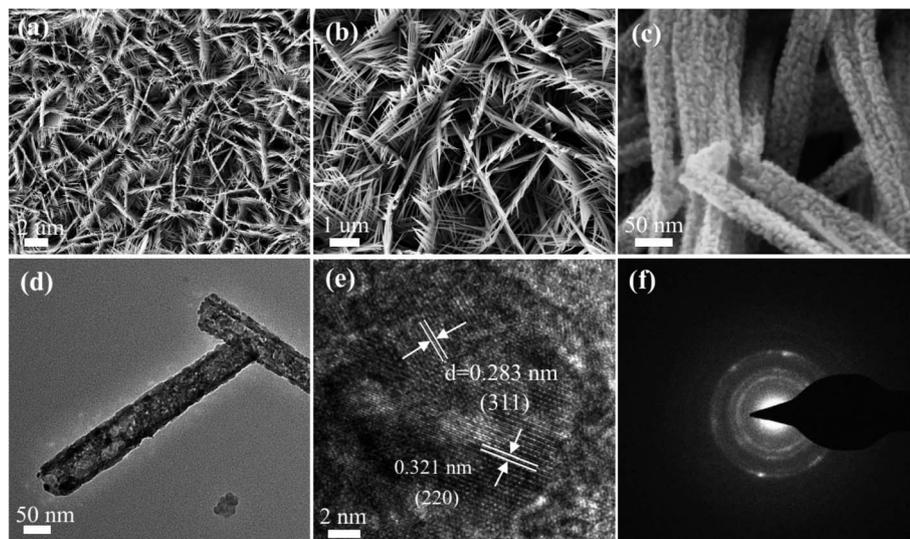
Fig. 3 SEM images of the as-fabricated  $\text{CoNi}_2\text{S}_4/\text{Ni}_3\text{S}_2$  nanowires. (a and b) Low magnification and (c) high magnification images. (d) TEM images. (e) HRTEM images. (f) SAED images.
