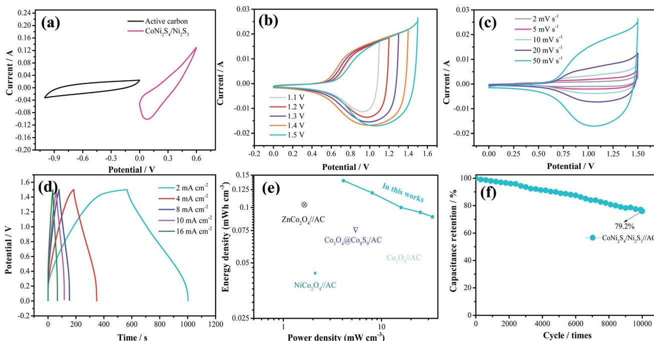
Fig. 5 Electrochemical performance characteristics of the as-fabricated device. (a) The CV comparison of CoNi<sub>2</sub>S<sub>4</sub>/Ni<sub>3</sub>S<sub>2</sub>//AC, (b) CV curves at different potential window, (c) CV curves, (d) GCD curves, (e) Ragone plots, (f) cycling stability measurements.
