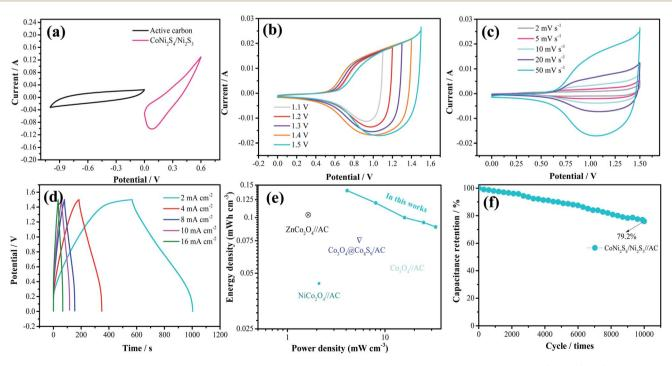
Fig. 5 Electrochemical performance characteristics of the as-fabricated device. (a) The CV comparison of  $CoNi_2S_4/Ni_3S_2/AC$ , (b) CV curves at different potential window, (c) CV curves, (d) GCD curves, (e) Ragone plots, (f) cycling stability measurements.
