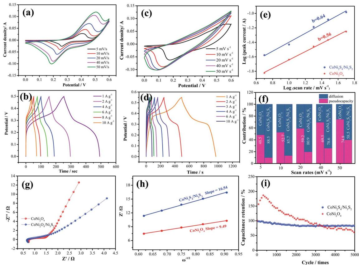
Fig. 4 Electrochemical performance measurements. (a) CV curves of  $\text{CoNi}_2\text{O}_4$ , (b) GCD curves of  $\text{CoNi}_2\text{O}_4$  samples, (c) CV curves of  $\text{CoNi}_2\text{S}_4/\text{Ni}_3\text{S}_2$ , (d) GCD curves of  $\text{CoNi}_2\text{S}_4/\text{Ni}_3\text{S}_2$ , (e)  $b$  values of two kinds of electrode materials, (f) capacitance contribution ratio, (g) Nyquist plots, (h)  $Z'$  as a function of  $\omega^{-1/2}$  plot in low frequency, (i) cycling stability tests.
