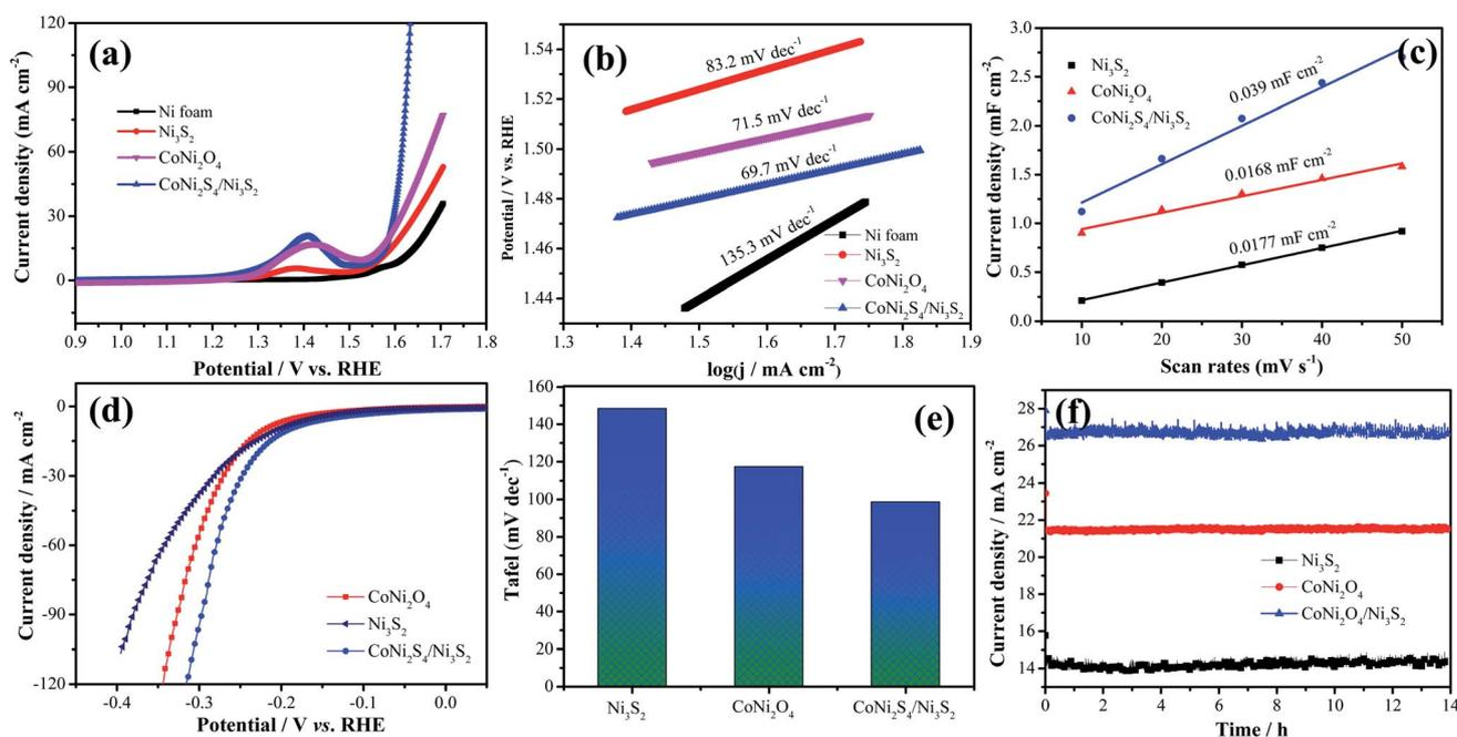
Fig. 7 (a–c) OER of the as-prepared catalysts, (a) LSV curves, (b) Tafel, (c) electric double layer capacitor value, (d) LSV curves for HER, (e) Tafel for HER, (f) cycle stability.
