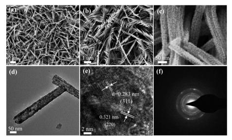
Fig. 3 SEM images of the as-fabricated  $CoNi_2S_4/Ni_3S_2$  nanowires. (a and b) Low magnification and (c) high magnification images. (d) TEM images. (e) HRTEM images. (f) SAED images.
