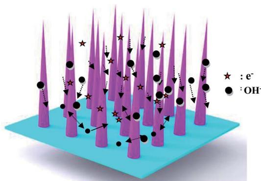
Fig. 6 Electrochemical mechanism diagram of the  $\text{CoNi}_2\text{S}_4/\text{Ni}_3\text{S}_2$  samples.
