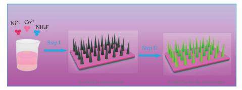
Fig. 1 Schematic illustration of the fabrication process of CoNi<sub>2</sub>S<sub>4</sub>/Ni<sub>3</sub>S<sub>2</sub> nanowires
