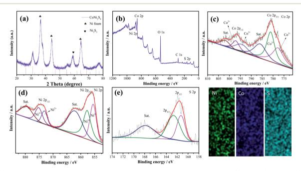
Fig. 2 (a) XRD pattern of the as-fabricated  $CoNi_2S_4/Ni_3S_2$  nanowires. (b) Survey spectra of the samples (c) Co 2p, (d) Ni 2p and (e) S 2p. (f) Elemental mapping.
