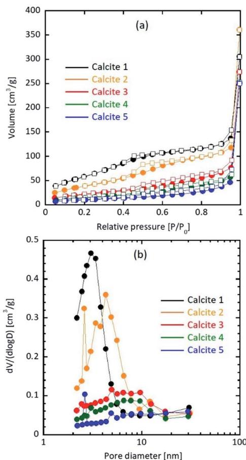
Fig. 1 (a) N<sub>2</sub> adsorption (circle)/desorption (square) isotherm and (b) pore size distribution of calcite particles.
