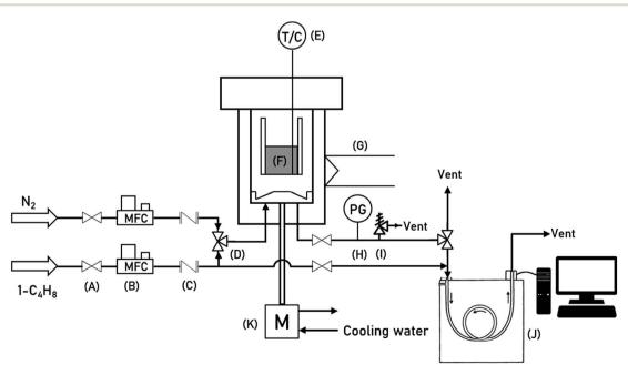
Fig. 1 A schematic of the experimental apparatus for 1-butene isomerization in the Berty-type reactor.
