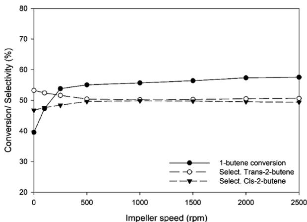
Fig. 4 Conversion of 1-butene and selectivity of *trans*-2-butene and *cis*-2-butene at different impeller speeds (rpm) at a temperature of 450 °C, inlet flow rate of 2.62 g h<sup>-1</sup> and 1 atm pressure.
