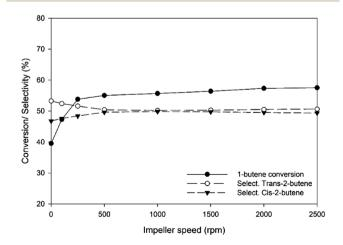
Fig. 4 Conversion of 1-butene and selectivity of *trans*-2-butene and *cis*-2-butene at different impeller speeds (rpm) at a temperature of 450  $^{\circ}$ C, inlet flow rate of 2.62 g h<sup>-1</sup> and 1 atm pressure.
