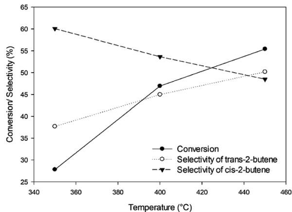
Fig. 7 The conversion of 1-butene and selectivities of *trans*-2-butene and *cis*-2-butene under pressure of 1 bar, inlet flow rate of  $2.62 \text{ g h}^{-1}$ , and impeller speed of 1500 rpm at different temperatures.
