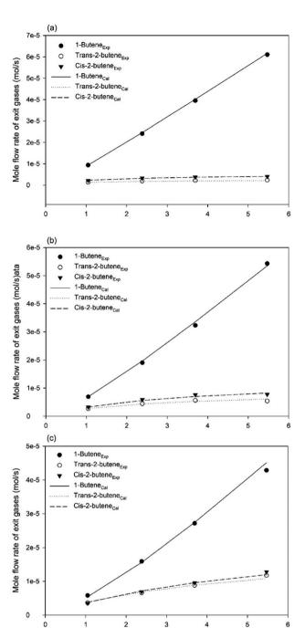
Fig. 9 Experimental and predicted molar flow rates of different gases for 1-butene isomerization under a pressure of 1 bar and impeller speed of 1500 rpm at different temperatures: (a)  $T=350~^{\circ}\text{C}$ , (b)  $T=400~^{\circ}\text{C}$ , and (c)  $T=450~^{\circ}\text{C}$ , respectively.
