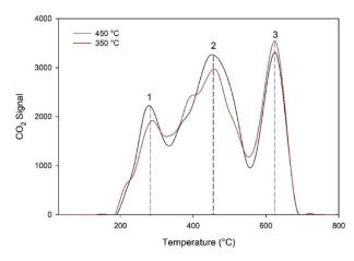
Fig. 3  $\,$  TPO profiles generated for the spent MgO catalyst at 350  $^{\circ}\text{C}$  and 450  $^{\circ}\text{C}.$
