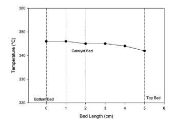
Fig. 6 The temperature profile of the catalytic bed in the Berty-type reactor at a set point temperature of 400  $^{\circ}$ C, pressure of 1 bar, and impeller speed of 1500 rpm.
