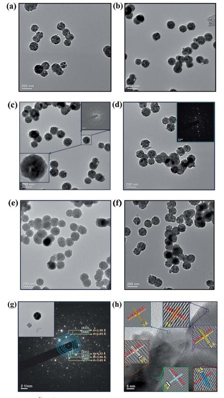
Fig. 6 HR-TEM Images of  $Y_2O_3$ :4 at%  $Eu^{3+}$ ,  $xLi^+$  (a) x=0.5 at%, (b) x=1 at%, (c) x=3 at%, (d) x=5 at%, (e) x=7 at%, (f) x=9 at% nanophosphors. (g) The magnified HR-TEM image and SAED pattern analysis of x=9 at% prepared crystalline sample. (h) Lattice fringes of x=9 at% samples corresponds to cubic yttrium(III) oxide ( $Y_2O_3$ ).
