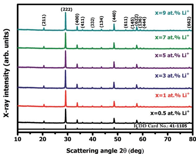
Fig. 1 X-ray diffraction (XRD) pattern of Y<sub>2</sub>O<sub>3</sub>:4 at% Eu<sup>3+</sup>, xLi<sup>+</sup> (x = 0.5, 1, 3, 5, 7, 9 at%) nanophosphors.
