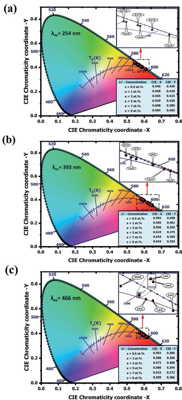
Fig. 10 The CIE 1931 chromaticity diagram of  $\text{Y}_2\text{O}_3:4$  at%  $\text{Eu}^{3+}$ ,  $x\text{Li}^+$  ( $x = 0.5, 1, 3, 5, 7, 9$  at%) nanophosphors excited by (a) 254 nm (b) 393 nm and (c) 466 nm, respectively.
