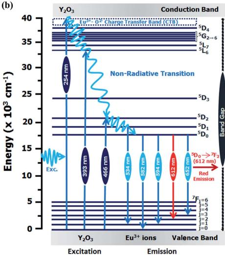
Fig. 9 (a) PL lifetime decay curves of  $Y_2O_3$ :4 at%  $Eu^{3+}$ ,  $xLi^+$  (x=0.5, 1, 3, 5, 7, 9 at%) nanophosphors. (b) Schematic energy level diagram for  $Y_2O_3$ :4 at%  $Eu^{3+}$ ,  $xLi^+$  (x=0.5, 1, 3, 5, 7, 9 at%) nanophosphors.
