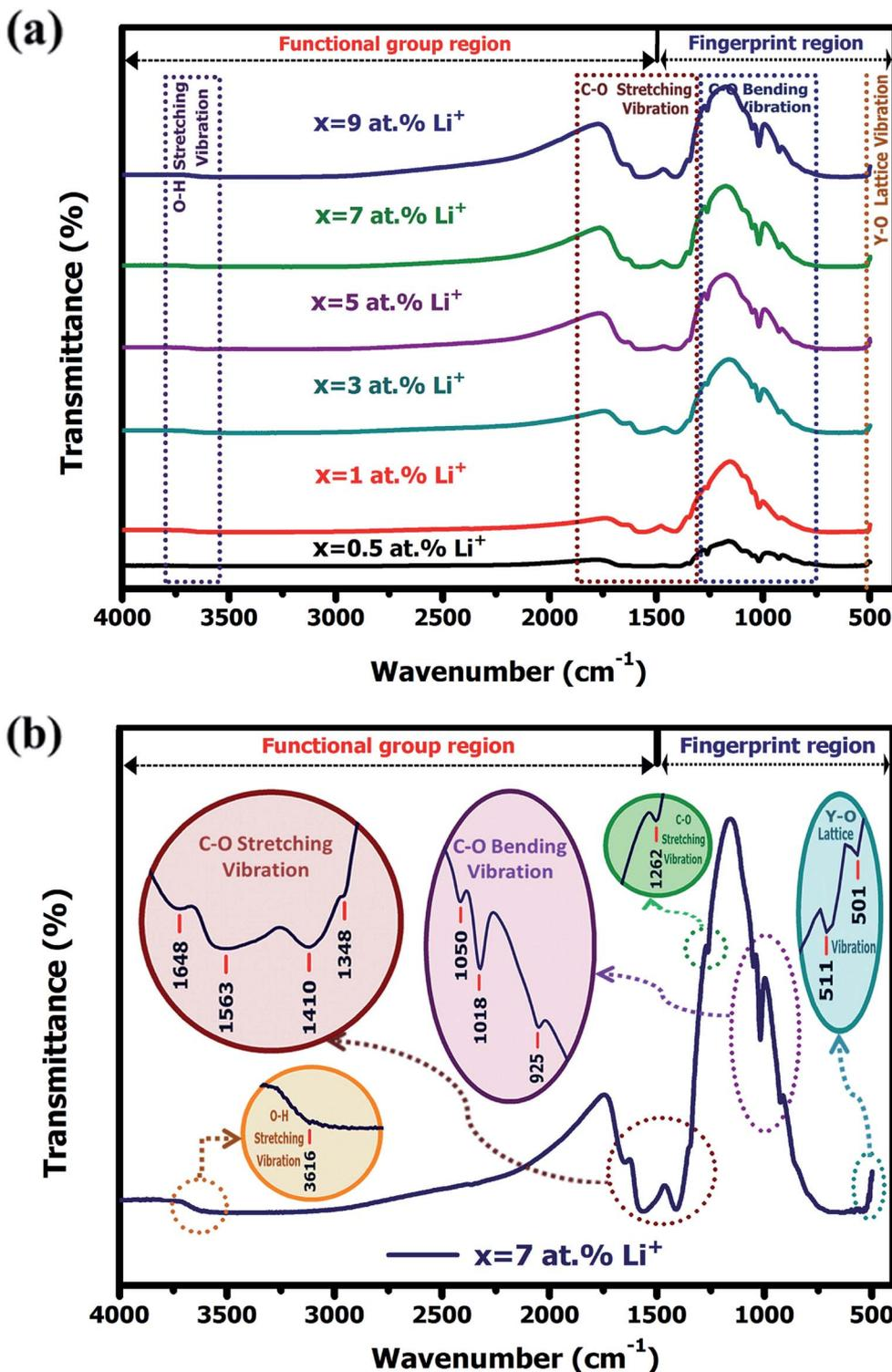
Fig. 5 (a) FTIR spectra of  $\text{Y}_2\text{O}_3:4 \text{ at}\% \text{Eu}^{3+}, x\text{Li}^+$  ( $x = 0.5, 1, 3, 5, 7, 9 \text{ at}\%$ ) nanophosphors. (b) The magnified FTIR spectra of  $\text{Y}_2\text{O}_3:4 \text{ at}\% \text{Eu}^{3+}, 7 \text{ at}\% \text{Li}^+$  nanophosphor.
