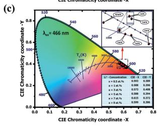
Fig. 10 The CIE 1931 chromaticity diagram of  $Y_2O_3$ :4 at% Eu<sup>3+</sup>, xLi<sup>+</sup> (x = 0.5, 1, 3, 5, 7, 9 at%) nanophosphors excited by (a) 254 nm (b) 393 nm and (c) 466 nm, respectively.
