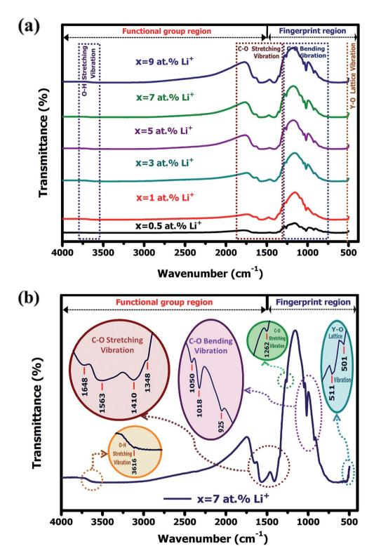
Fig. 5 (a) FTIR spectra of  $Y_2O_3$ :4 at%  $Eu^{3+}$ ,  $xLi^+$  (x=0.5,1,3,5,7,9 at%) nanophosphors. (b) The magnified FTIR spectra of  $Y_2O_3$ :4 at%  $Eu^{3+}$ , 7 at%  $Li^+$  nanophosphor.
