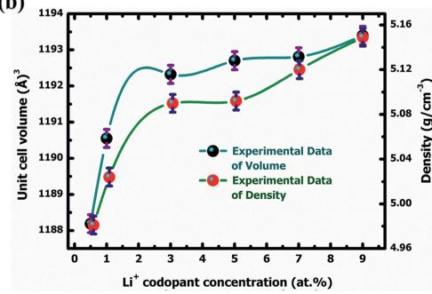
Fig. 2 W-H plot of  $Y_2O_3$ :4 at%  $Eu^{3+}$ ,  $xLi^+$  (a) x=3 at% nanophosphor (b) variation of unit cell volume and density with  $Li^+$  codoping concentration.
