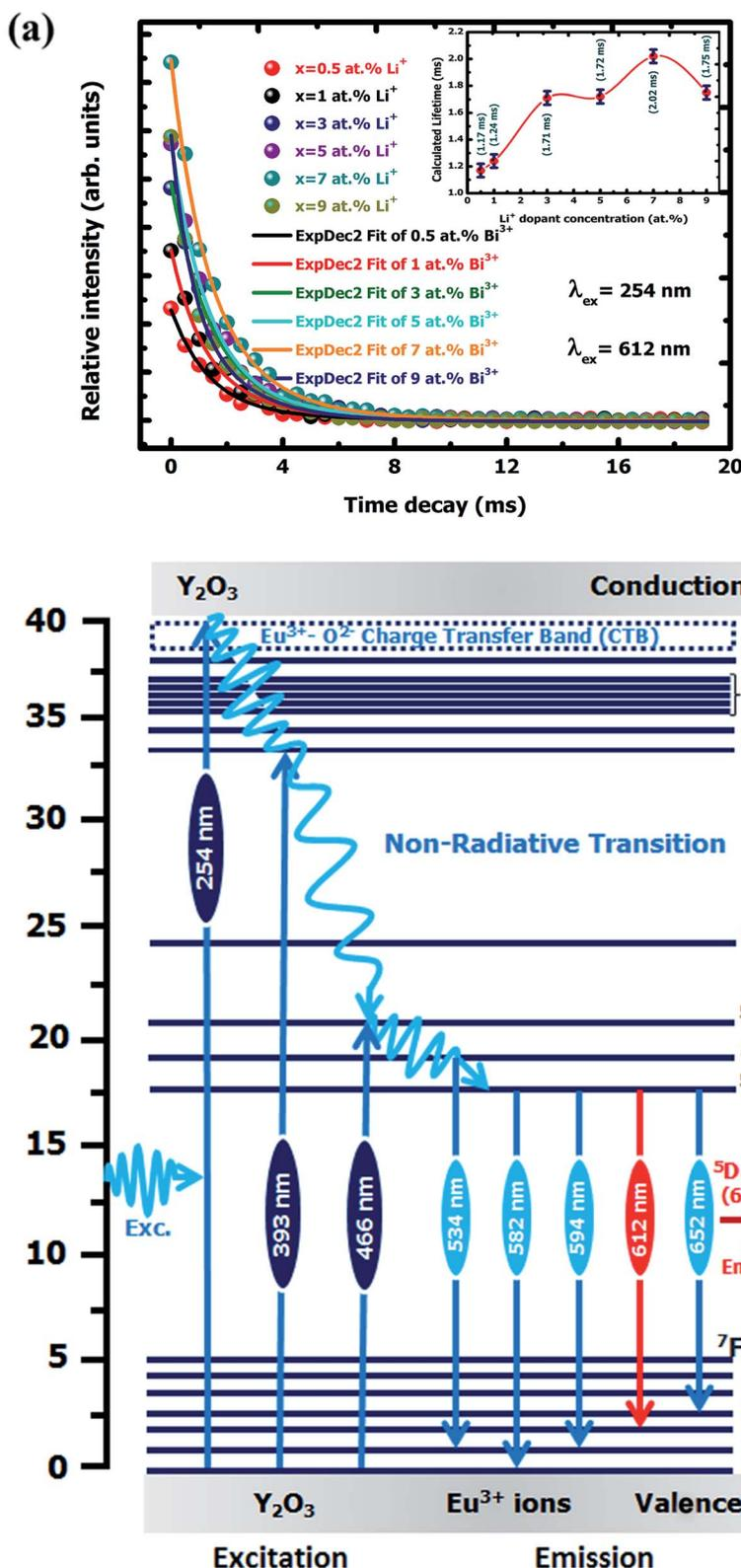
Fig. 9 (a) PL lifetime decay curves of  $\text{Y}_2\text{O}_3:4 \text{ at}\% \text{Eu}^{3+}, x\text{Li}^+$  ( $x = 0.5, 1, 3, 5, 7, 9 \text{ at}\%$ ) nanophosphors. (b) Schematic energy level diagram for  $\text{Y}_2\text{O}_3:4 \text{ at}\% \text{Eu}^{3+}, x\text{Li}^+$  ( $x = 0.5, 1, 3, 5, 7, 9 \text{ at}\%$ ) nanophosphors.
