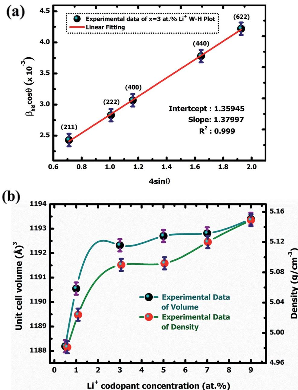
Fig. 2 W–H plot of  $Y_2O_3:4 \text{ at}\% \text{ Eu}^{3+}$ ,  $x\text{Li}^+$  (a)  $x = 3 \text{ at}\%$  nanophosphor (b) variation of unit cell volume and density with  $\text{Li}^+$  codoping concentration.
