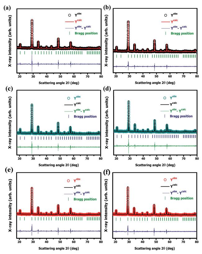
Fig. 3 Rietveld refined XRD pattern of  $Y_2O_3$ :4 at%  $Eu^{3+}$ ,  $xLi^+$  nanophosphors (a) x=0.5 at%, (b) x=1 at% (c) x=3 at%, (d) x=5 at%, (e) x=7 at%, and (f) x=9 at%, respectively.
