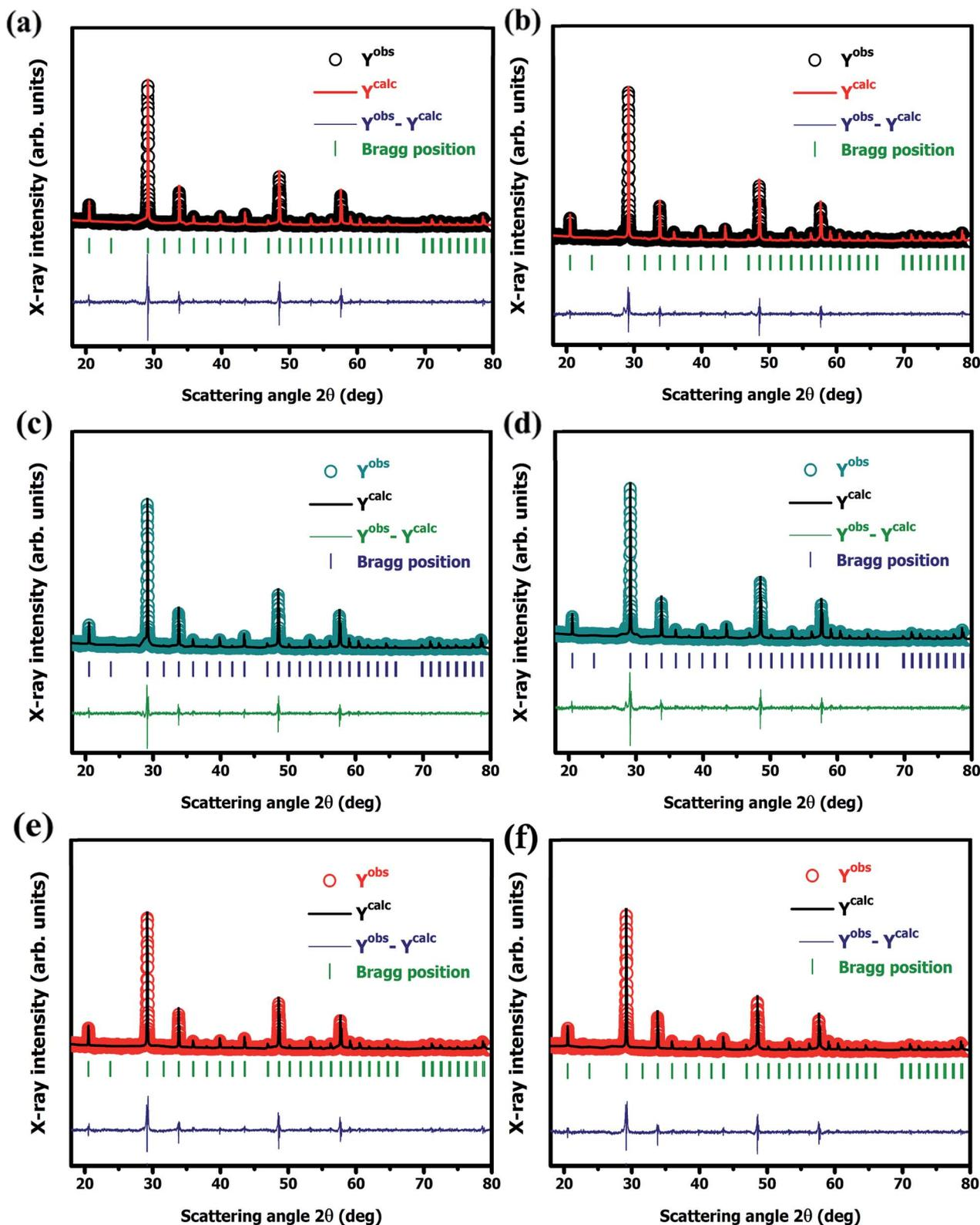
Fig. 3 Rietveld refined XRD pattern of  $\text{Y}_2\text{O}_3:4 \text{ at}\% \text{Eu}^{3+}, x\text{Li}^+$  nanophosphors (a)  $x = 0.5 \text{ at}\%$ , (b)  $x = 1 \text{ at}\%$  (c)  $x = 3 \text{ at}\%$ , (d)  $x = 5 \text{ at}\%$ , (e)  $x = 7 \text{ at}\%$ , and (f)  $x = 9 \text{ at}\%$ , respectively.
