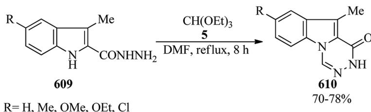
Scheme 182 The formation of new 8-substituted-10-methyl-1,2-dihydro-1-oxo-1,2,4-triazino[4,5-a]indoles.
