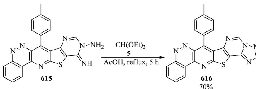
Scheme 185 The synthesis of 7-(*p*-tolyl)-1,2,4-triazolo[4''',3''':1'',6'']pyrimido[4'',5'':4',5']thieno[3',2':5,6]pyrido[3,2-*c*]cinnoline.
