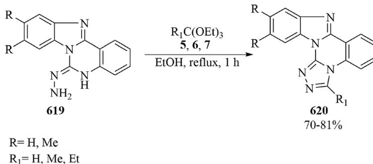
Scheme 187 Obtaining new benzimidazo[1,2-c][1,2,4]triazolo[4,3-a]quinazolines.
