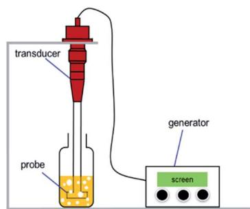
Fig. 1 Schematic configuration diagram of ultrasonic system, including an ultrasonic generator, a high-power ultrasonic transducer, and an ultrasonic probe.
