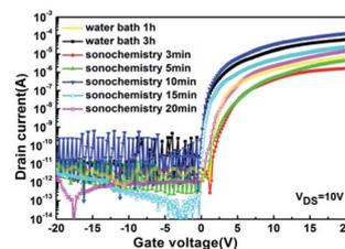
Fig. 7 Transfer characteristics ( $I_{DS}-V_{GS}$ ) of the WZTO TFT device with different treatments of precursor solution.
