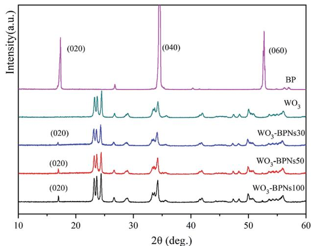
Fig. 1 XRD patterns of bulk BP, WO<sub>3</sub> and WO<sub>3</sub>-BPNs composites.
