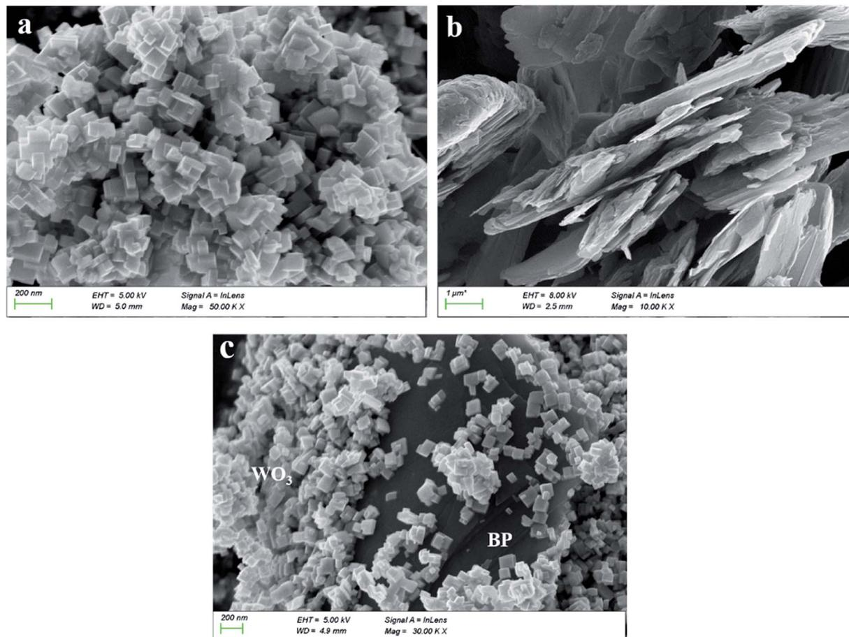
Fig. 2 SEM images of WO<sub>3</sub> (a), BPNs (b) and WO<sub>3</sub>-BPNs50 composites (c).
