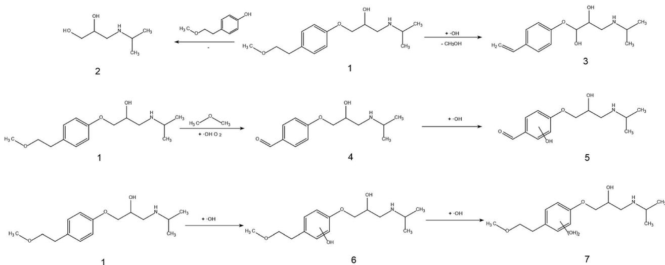
Fig. 14 Tentative pathways for the photocatalytic degradation of MET using WO<sub>3</sub>-BPNs.
