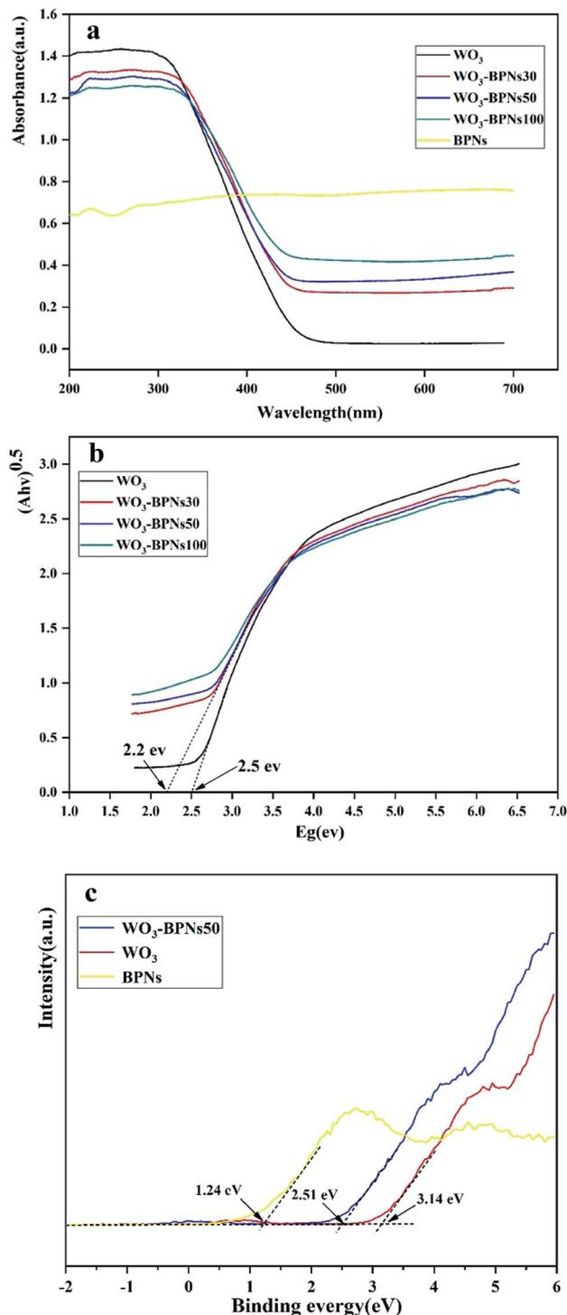
Fig. 5 UV-vis diffuse reflectance spectra of  $\text{WO}_3$  and  $\text{WO}_3$ -BPNs (a), and plot of the  $(ah\nu)^{0.5}$  versus  $h\nu$  (b), VB XPS spectra of  $\text{WO}_3$ , BPNs and  $\text{WO}_3$ -BPNs50 (c).
