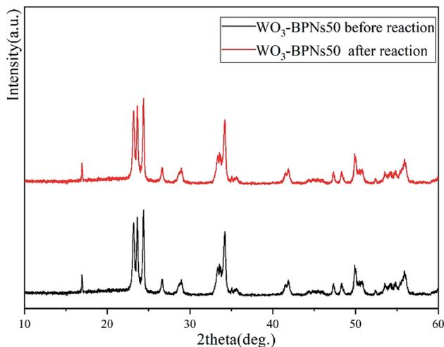
Fig. 10 XRD patterns of the WO<sub>3</sub>-BPNs50 sample before reaction and after photocatalytic reaction under visible-light.
