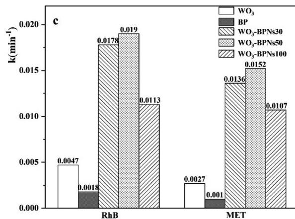
Fig. 8 Photocatalytic degradation of RhB (a) and MET (b) using WO<sub>3</sub>, BP and WO<sub>3</sub>-BPNs samples. (c) First order rate constant  $k$  (min<sup>-1</sup>) of all samples for RhB and MET.
