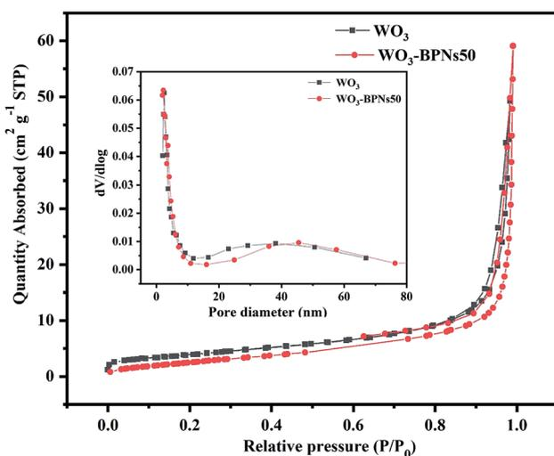
Fig. 7 N<sub>2</sub> absorption-desorption isotherms and corresponding pore size distribution curves for WO<sub>3</sub> and WO<sub>3</sub>-BPNs50.
