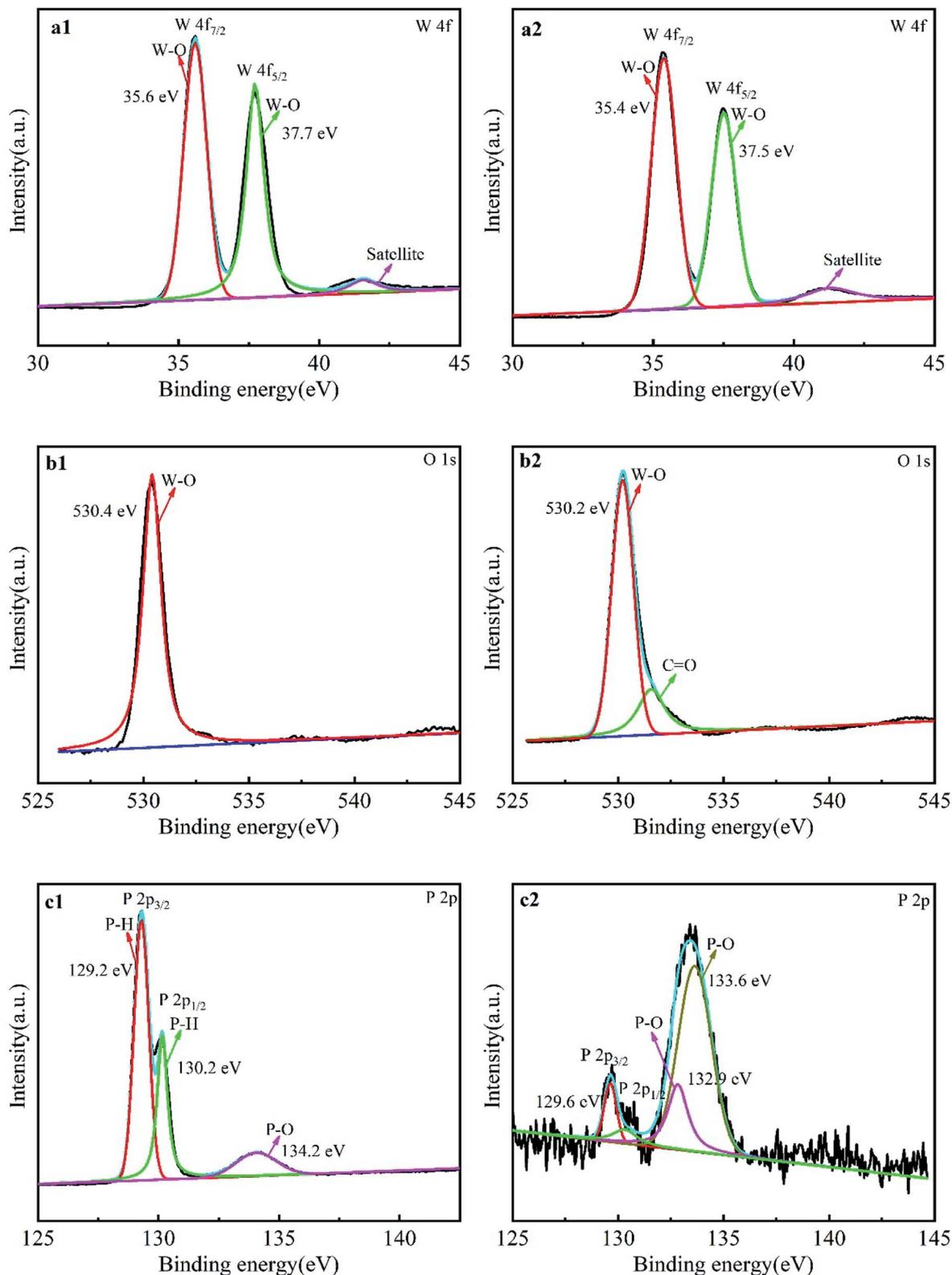
Fig. 4 XPS spectra for W 4f of WO<sub>3</sub> (a1) and WO<sub>3</sub>-BPNs50 (a2), O 1s of WO<sub>3</sub> (b1) and WO<sub>3</sub>-BPNs (b2), and P 2p of BP (c1) and WO<sub>3</sub>-BPNs (c2).
