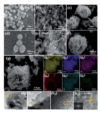
Fig. 3 SEM images of ZCO@C $_3$ N $_4$  (a and d), ZCO@C $_3$ N $_4$ -S (b and e), ZCO@C $_3$ N $_4$ -B (c and f); (g-g $_6$ ) SEM images and the corresponding SEM-EDS elemental mapping of Zn, Co, O, C, B and N for the ZCO@C $_3$ N $_4$ -B; (h-h $_3$ ) HRTEM images of the ZCO@C $_3$ N $_4$ -B.
