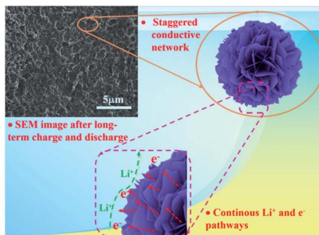
Fig. 8 Mechanism explanations of the excellent electrochemical performance of the nanoflower ZCO@C<sub>3</sub>N<sub>4</sub>-B electrode.
