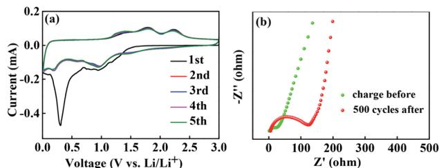
Fig. 7 (a) Cyclic voltammetry curves during the initial five cycles for the ZCO@C<sub>3</sub>N<sub>4</sub>-B electrode; (b) electrochemical impedance of the ZCO@C<sub>3</sub>N<sub>4</sub>-B electrodes after 500 cycles and the charge before.
