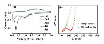
Fig. 7 (a) Cyclic voltammetry curves during the initial five cycles for the ZCO@C $_3$ N $_4$ -B electrode; (b) electrochemical impedance of the ZCO@C $_3$ N $_4$ -B electrodes after 500 cycles and the charge before.
