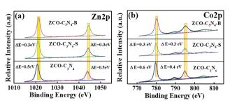
Fig. 5 (a and b) XPS spectra comparison of the Zn 2p and Co 2p spectra of  $ZCO@C_3N_4$ ,  $ZCO@C_3N_4$ -S and  $ZCO@C_3N_4$ -B.
