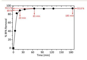
Fig. 4 Percentage of BPA removal at 25 °C, at a contact time ranging from 0 to 180 min (initial concentration of 80.9 mg  $L^{-1}$ ).
