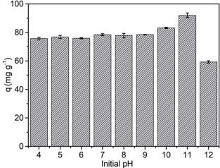
Fig. 2 Effect of the initial pH on the adsorption capacity of BPA. Conditions: 25 °C, initial concentration 100 mg L<sup>-1</sup>, contact time 2 h and adsorbent mass 1.0 g  $L^{-1}$  (see Fig. S2 and Table S1†).
