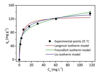
Fig. 6 Adsorption Langmuir and Freundlich isotherms for BPA adsorbed by silica nanoparticles. Conditions: 25 °C, contact time 1 h and adsorbent mass 1.0 g  $\rm L^{-1}$  (see Fig. S7, Table S6 and S7†).
