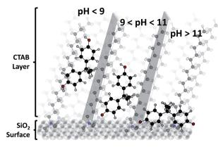
Fig. 3 Scheme illustrating the organization of BPA on the surface of MSN-CTAB at different pH values.
