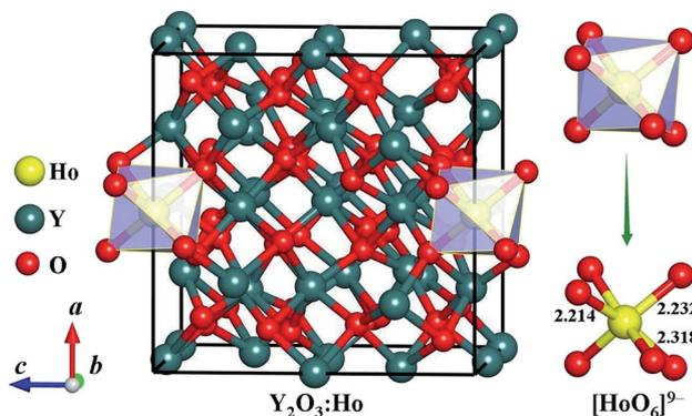
Fig. 1 Crystal structure and [HoO<sub>6</sub>]<sup>9–</sup> local unit of the ground-state Ho<sup>3+</sup>-doped Y<sub>2</sub>O<sub>3</sub>. The bond lengths are in the unit of Å.
