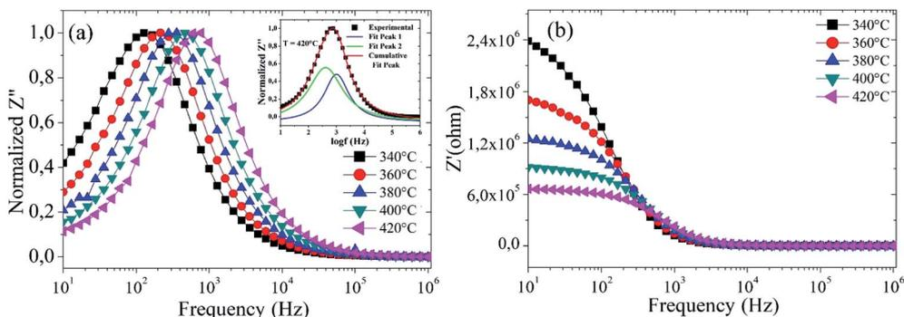
**Fig. 7** Variation of (a) the imaginary part ( $Z''$ ), and (b) the real part ( $Z'$ ) of impedance with frequency at different temperatures for Ba<sub>5</sub>CaTi<sub>1.94</sub>-Zn<sub>0.06</sub>Nb<sub>8</sub>O<sub>30</sub> ceramic.
