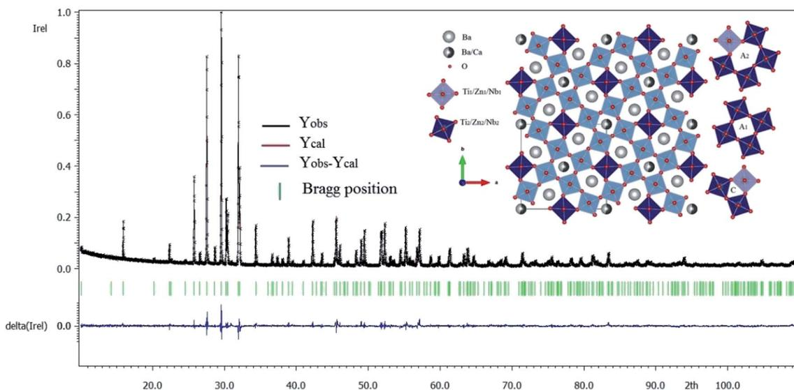
Fig. 1 X-ray diffraction refinement for  $\text{Ba}_5\text{CaTi}_{1.94}\text{Zn}_{0.06}\text{Nb}_8\text{O}_{30}$  powder, and representation of the TTB structure of  $\text{Ba}_5\text{CaTi}_{1.94}\text{Zn}_{0.06}\text{Nb}_8\text{O}_{30}$  along the "c" axis.
