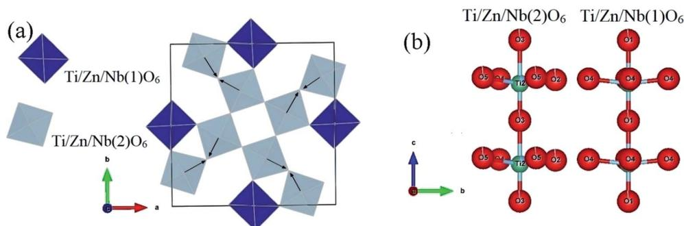
Fig. 2 (a) Polyhedral representation of Ba<sub>5</sub>CaTi<sub>1.94</sub>Zn<sub>0.06</sub>Nb<sub>8</sub>O<sub>30</sub> ceramic along the "c" axis. (b) Representation describing the distortions of the two kinds of octahedra in Ba<sub>5</sub>CaTi<sub>1.94</sub>Zn<sub>0.06</sub>Nb<sub>8</sub>O<sub>30</sub> ceramic along the "a" axis.
