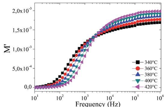
**Fig. 8** Real part of the module as a function of frequency for Ba<sub>5</sub>CaTi<sub>1.94</sub>Zn<sub>0.06</sub>Nb<sub>8</sub>O<sub>30</sub> ceramic.
