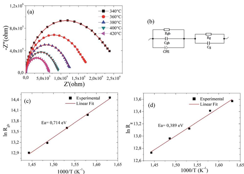
Fig. 5 (a) Nyquist plot fitted with an equivalent circuit for  $\text{Ba}_5\text{CaTi}_{1.94}\text{Zn}_{0.06}\text{Nb}_8\text{O}_{30}$  ceramic at different temperatures. (b) Electrical equivalence circuit for the modeling of the impedance data. Arrhenius plot of the data obtained from the results of impedance circles; (c) for grain boundaries, and (d) for grains.
