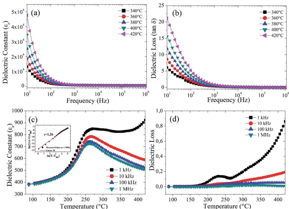
Fig. 4 (a) and (b) Frequency dependence of dielectric properties of  $\text{Ba}_5\text{CaTi}_{1.94}\text{Zn}_{0.06}\text{Nb}_8\text{O}_{30}$  ceramic ranging from 10 Hz to 1 MHz. (c) and (d) Temperature dependence of the dielectric constant ( $\epsilon_r$ ) and dielectric loss ( $\tan \delta$ ) for  $\text{Ba}_5\text{CaTi}_{1.94}\text{Zn}_{0.06}\text{Nb}_8\text{O}_{30}$  ceramic respectively.
