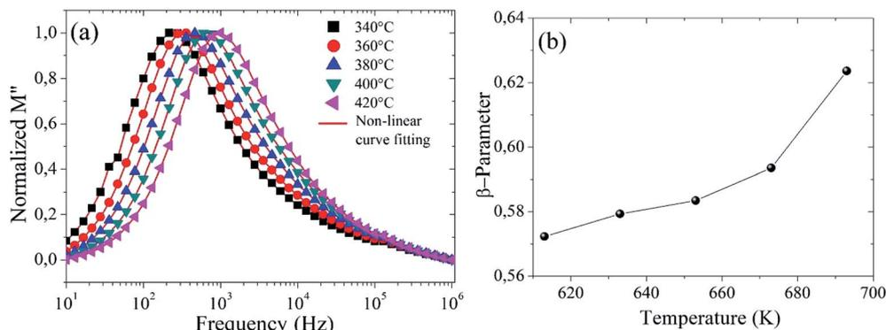
Fig. 9 (a) Imaginary part of the module as a function of frequency, and (b) the plot of  $\beta$ -parameter versus temperature for  $\text{Ba}_5\text{CaTi}_{1.94}\text{Zn}_{0.06}\text{Nb}_8\text{O}_{30}$  ceramic.
