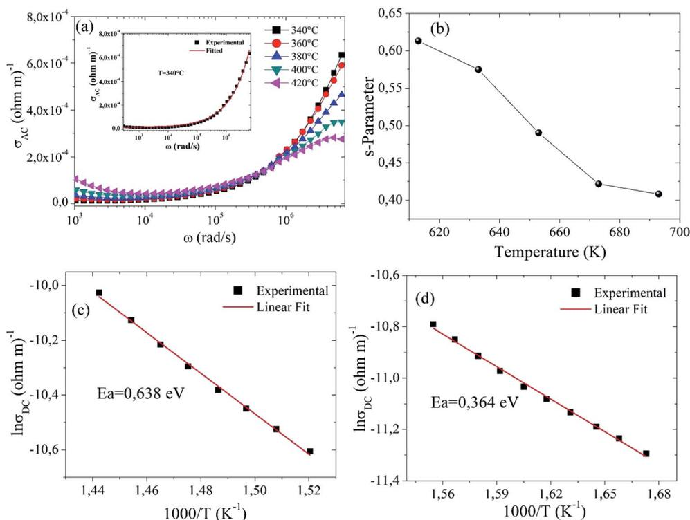
Fig. 6 (a) AC conductivity as a function of frequency. (b) Variation of *s*-parameter with temperature for  $\text{Ba}_5\text{CaTi}_{1.94}\text{Zn}_{0.06}\text{Nb}_8\text{O}_{30}$  ceramic. (c), and (d)  $\ln \sigma_{\text{DC}}$  as a function of  $10^3/T$  for  $\text{Ba}_5\text{CaTi}_{1.94}\text{Zn}_{0.06}\text{Nb}_8\text{O}_{30}$  ceramic for grain boundaries, and for grains at 1 kHz respectively.
