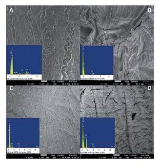
Fig. 7 EDX in SEM images of (A) calcium alginate beads; (B) Ca-Alg-GA-PEI beads; (C) Ca-Alg-GA-PEI beads after biosorption of [As(III)]; (D) Ca-Alg-GA-PEI beads after biosorption of [As(V)].
