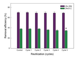
Fig. 10 Removal efficiency of Ca-Alg-GA-PEI after five desorption/adsorption cycles. Asterisk denotes significant difference (p < 0.05) between the cycles of the same oxyanion.
