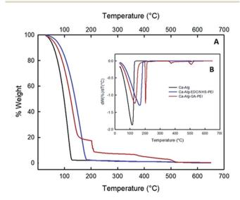
Fig. 5 Thermogravimetric/derivative thermogravimetry analysis for calcium alginate beads functionalized with polyethyleneimine (PEI). Crosslinking agents EDC/NHS: 1-ethyl-3-(3-dimethylaminopropyl) carbodiimide/N-hydroxysuccinimide; GA: glutaraldehyde.
