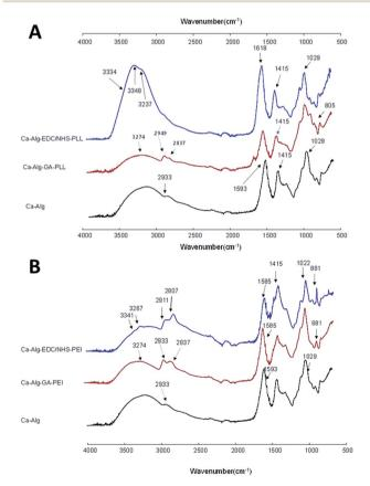
Fig. 3 Attenuated total reflectance Fourier transform infrared spectroscopy for calcium alginate beads functionalized with (A) poly-L-lysine and (B) polyethylenimine.
