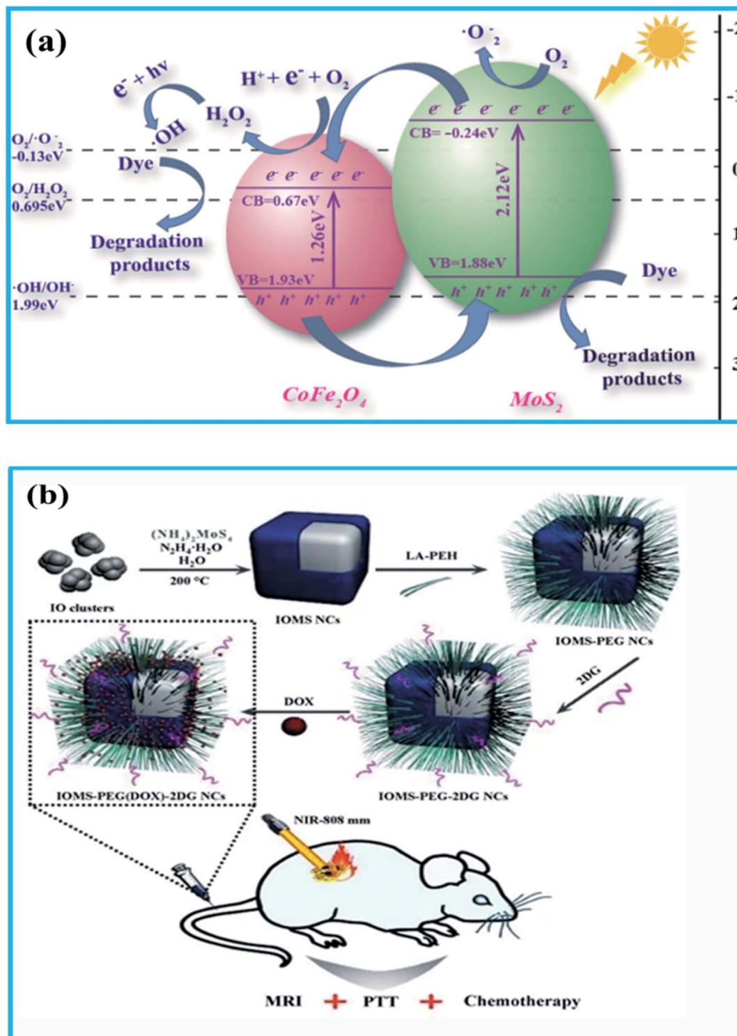
Fig. 12 (a) A possible mechanism explaining the photocatalytic activity of  $\text{CoFe}_2\text{O}_4/\text{MoS}_2$  heterojunctions for the degradation of CR under visible light irradiation. (b) A schematic illustration of the fabrication process of IOMS-PEG(DOX)-2DG NCs for MRI-guided chemo-photothermal cancer therapy (reprinted with permission from ref. 249 and 258; copyright: 2018, Elsevier Ltd.).
