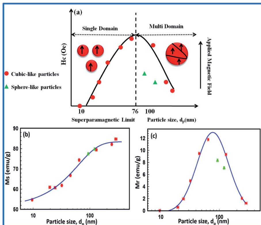
Fig. 2 The particle size dependence of (a) coercivity ( $H_c$ ); (b) saturation magnetization ( $M_s$ ); and (c) remanent magnetization ( $M_r$ ) for cube-like and sphere-like morphologies of Fe<sub>3</sub>O<sub>4</sub> nanoparticles (reprinted with permission from ref. 73; copyright: 2017, Springer Nature).
