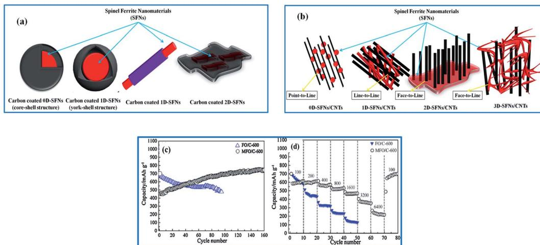
Fig. 6 The various hybrid designs of (a) carbon-coated SFNs and (b) CNTs/SFNs. (c and d) The cycling performances at a current density of  $100 \text{ mA g}^{-1}$  and rate capabilities of MFO/C and FO/C (reprinted with permission from ref. 101; copyright: 2013, Elsevier Ltd).
