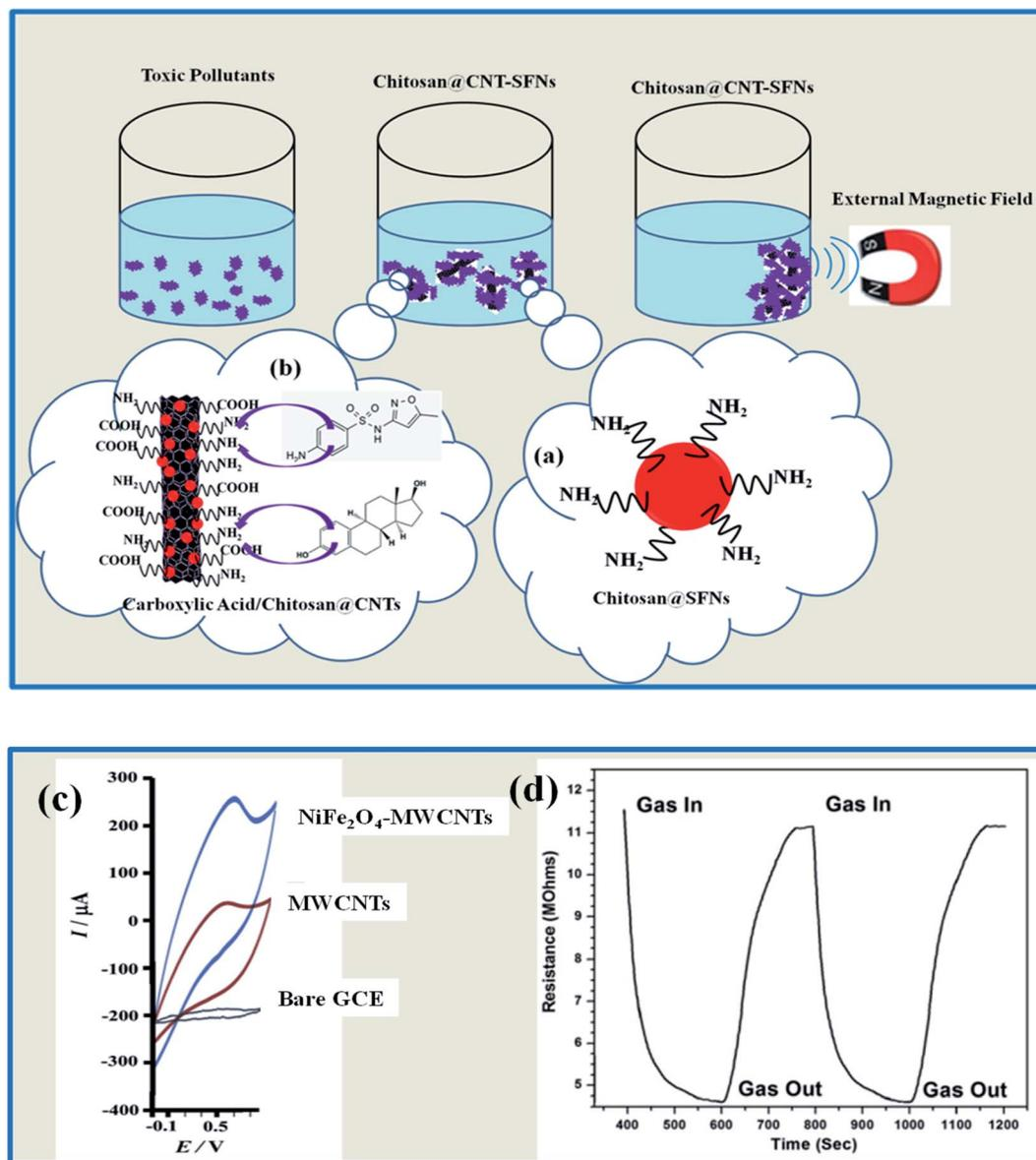
Fig. 8 (a and b) The surface modifications of SFNs and CNTs for pollutant removal applications. (c) The voltammetric responses of various sensor electrodes to totalol. (d) The response of a NiFe<sub>2</sub>O<sub>4</sub>-MWCNT thin film towards 100 ppm H<sub>2</sub>S at 300 °C (reprinted with permission from ref. 136 and 138; copyright: 2013 and 2014, Elsevier Ltd, respectively).
