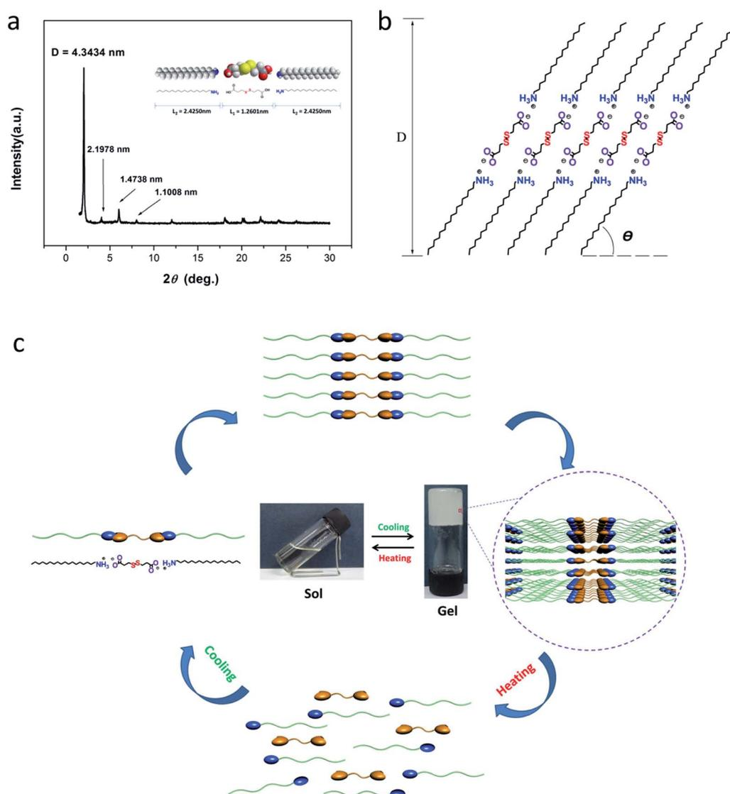
Fig. 6 (a) XRD pattern of DPA-R<sub>18</sub> xerogel (7.49 wt%, solvent: DMSO; inset: CPK space-filling models of DPA and R<sub>18</sub>-NH<sub>2</sub>); (b) local microstructure of aggregates in DPA-R<sub>18</sub> organogel; (c) schematic representation of self-assembly mechanism.
