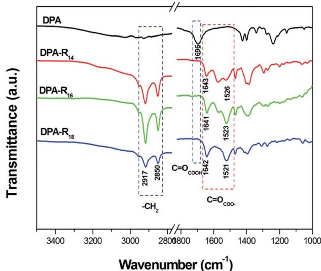
Fig. 5 FT-IR spectra of DPA and the xerogels formed from DPA-R<sub>14</sub> (4.25 wt%), DPA-R<sub>16</sub> (2.31 wt%) or DPA-R<sub>18</sub> (1.67 wt%) in DMSO, respectively.
