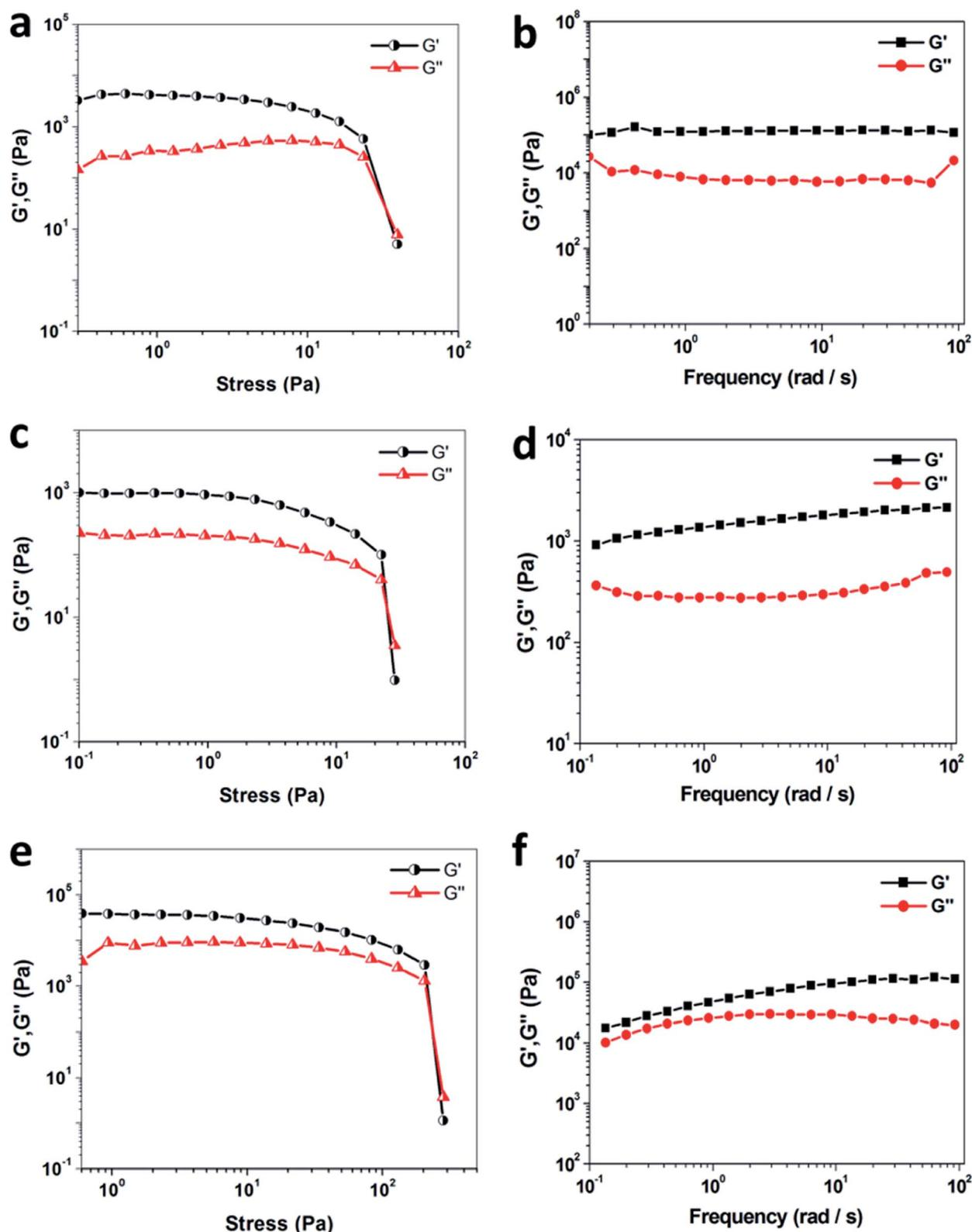
Fig. 4 Rheological behaviors of the organogels formed from DPA-R<sub>18</sub> in DMF, chlorobenzene and isopropyl ether, respectively: (a, c and e) strain sweep results and (b, d and f) frequency sweep results at a constant strain of 5 Pa.
