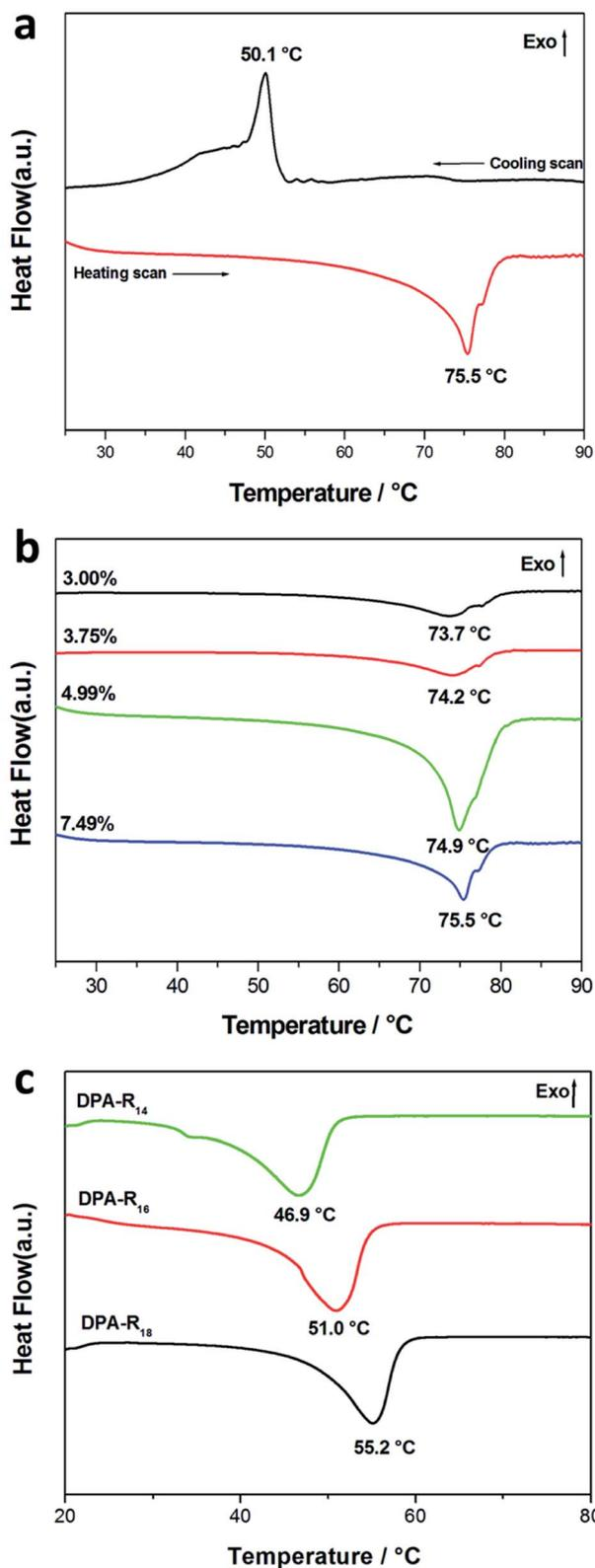
Fig. 2 DSC thermograms of the gels formed from (a) DPA- $R_{18}$  in DMSO (7.49 wt%), (b) DPA- $R_{18}$  in DMSO with different gelator concentrations (wt%) and (c) DPA- $R_{14}$ , DPA- $R_{16}$  and DPA- $R_{18}$  in cyclohexane (3.75 wt%).
