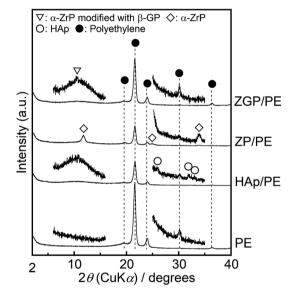
Fig. 3 GI-XRD patterns of the prepared substrates.
