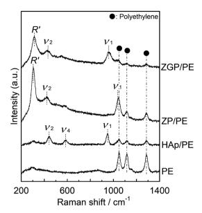
Fig. 4 Raman spectra of the prepared substrates.
