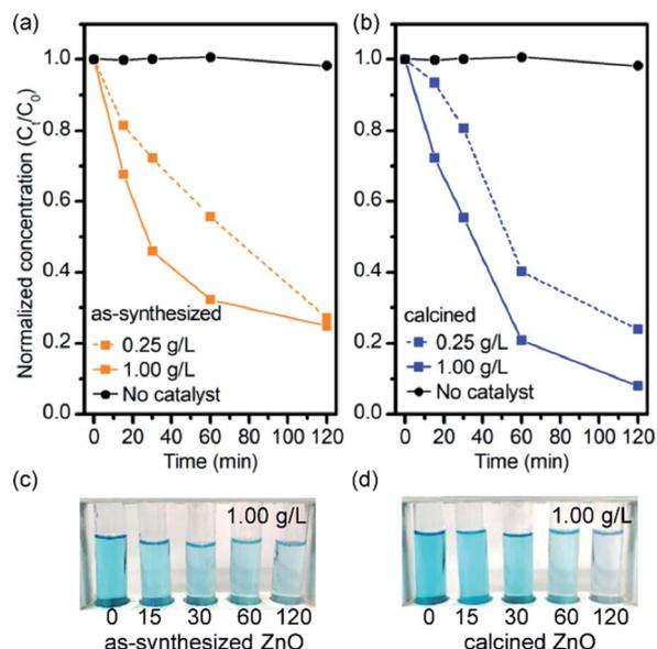
Fig. 6 Piezo-promoted photodegradation efficiency of MB solutions in 0.25 g L<sup>-1</sup> and 1.00 g L<sup>-1</sup> mixtures of (a) as-synthesized ZnO<sub>TW-0.20</sub> and (b) calcined ZnO<sub>TW-0.20</sub> under ultrasonic radiation and UV light with their optical images of MB in 1.00 g L<sup>-1</sup> mixtures solution in (c) and (d), respectively.
