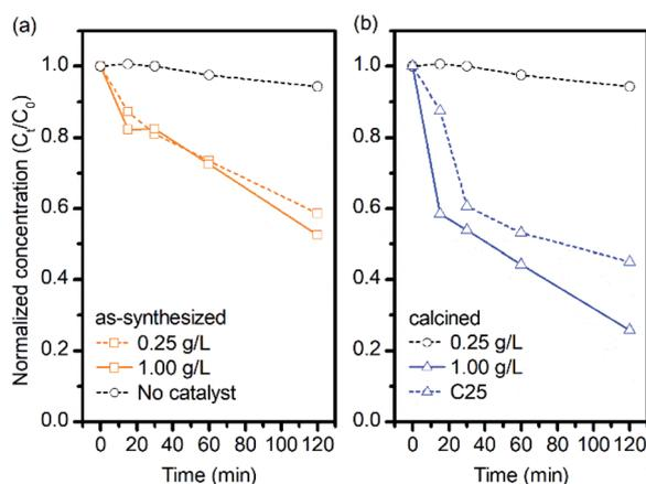
Fig. 3 Photodegradation efficiency of MB solutions in  $0.25 \text{ g L}^{-1}$  and  $1.00 \text{ g L}^{-1}$  mixtures of (a) as-synthesized  $\text{ZnO}_{\text{TW-0.20}}$  and (b) calcined  $\text{ZnO}_{\text{TW-0.20}}$  under exposure to UV light.
