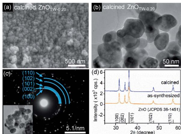
Fig. 5 (a) A SEM image of the calcined ZnO<sub>TW-0.20</sub>, (b) a bright field TEM image taken from the calcined ZnO<sub>TW-0.20</sub>, (c) a diffraction pattern of a group of calcined ZnO<sub>TW-0.20</sub> particles shown in the image inset (d) XRD patterns of calcined ZnO<sub>TW-0.20</sub> and as-synthesized ZnO<sub>TW-0.20</sub>.
