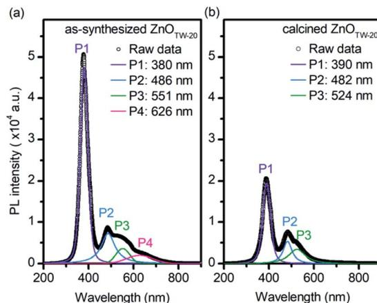
Fig. 4 Room temperature PL spectra of (a) as-synthesized  $\text{ZnO}_{\text{TW-0.20}}$  and (b) calcined  $\text{ZnO}_{\text{TW-0.20}}$ . The experimental raw data and the fitted curves are represented by open circles and solid lines, respectively.
