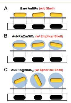
Fig. 2 (A) Schematic of bare AuNRs deposited on a glass slide. Their projected lengths are almost the same. (B) Schematic of elliptical AuNRs@mSiO2 particles and their projections on a glass slide. (C) Schematic of spherical AuNRs@mSiO2 particles with their AuNR cores randomly oriented in the shell. Their projected lengths depend on their spatial orientations, which are freely available in 3D space.
