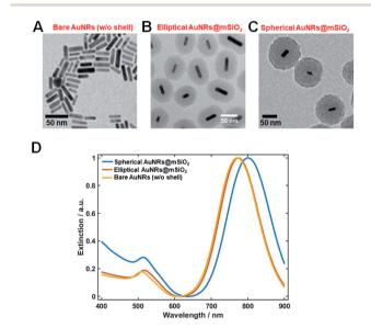
Fig. 1 (A–C) TEM images of (A) bare AuNRs, (B) elliptical AuNRs@mSiO $_2$  (red curve), and (C) spherical AuNRs@mSiO $_2$  (blue curve). (D) Overlaid UV-vis extinction spectra of bare AuNRs (yellow curve), elliptical AuNRs@mSiO $_2$  (red curve), and spherical AuNRs@mSiO $_2$  (blue curve). The anisotropic AuNRs yielded two distinct LSPR peaks.
