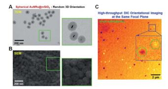
Fig. 3 (A) TEM image of spherical AuNRs@mSiO<sub>2</sub> with randomly oriented AuNR cores inside the silica shell. (B) SEM image of spherical AuNRs@mSiO<sub>2</sub> particles, and (C) DIC image of AuNRs@mSiO<sub>2</sub> particles, showing their different orientations on the same focal plane. The color image was generated in ImageJ for better demonstration of bright and dark DIC images of AuNRs@mSiO<sub>2</sub>. Note that high-throughput detection is possible.
