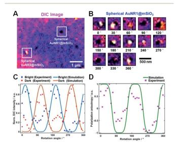
Fig. 4 (A) DIC image of spherical AuNRs@mSiO<sub>2</sub>. (B) DIC images of spherical AuNR1@mSiO<sub>2</sub> captured at different rotational angles (interval =  $30^{\circ}$ ). (C) Dark and bright intensities of spherical AuNR1@mSiO<sub>2</sub> as functions of rotation angle. (D) DIC polarization anisotropy computed from the dark and bright intensities of the spherical AuNR1@mSiO<sub>2</sub>.
