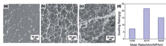
Fig. 5 SEM images of IPN-pNIPAm@Fe<sub>2</sub>O<sub>3</sub>-SiO<sub>2</sub> nanogels with different molar ratio: (a) AAm/NIPAm (10/90)-1.2%BIS, (b) AAm/NIPAm (30/70)-1.2%BIS, (c) AAm/NIPAm (50/50)-1.2%BIS, and (d) the effect of molar ratio (AAm/NIPAm) on the swelling property of IPN-pNIPAm@Fe<sub>2</sub>O<sub>3</sub>-SiO<sub>2</sub> nanogels.
