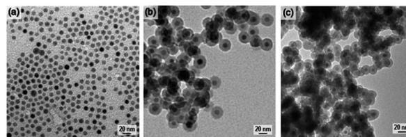
Fig. 2 TEM images of (a) Fe<sub>2</sub>O<sub>3</sub> magnetic nanoparticles, (b) Fe<sub>2</sub>O<sub>3</sub>-SiO<sub>2</sub> magnetic nanoparticles, and (c) AAm-Fe<sub>2</sub>O<sub>3</sub>-SiO<sub>2</sub> magnetic nanoparticles.
