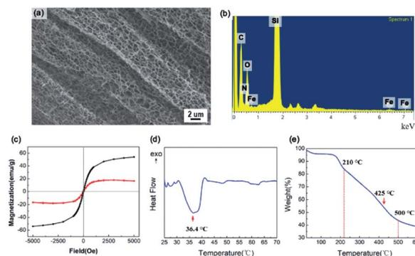
Fig. 3 (a) SEM image and (b) EDX of IPN-pNIPAm@Fe<sub>2</sub>O<sub>3</sub>-SiO<sub>2</sub> nanogels, (c) the magnetization curve of Fe<sub>2</sub>O<sub>3</sub> magnetic nanoparticles (black) and IPN-pNIPAm@Fe<sub>2</sub>O<sub>3</sub>-SiO<sub>2</sub> nanogels (red), (d) DSC curve, and (e) TGA curve of IPN-pNIPAm@Fe<sub>2</sub>O<sub>3</sub>-SiO<sub>2</sub> nanogels.
