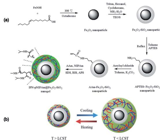
Fig. 1 (a) Schematic illustration for the preparation of IPN-pNIPAm@Fe<sub>2</sub>O<sub>3</sub>-SiO<sub>2</sub> nanogels, and (b) the dynamic mechanism of the phase transition of IPN-pNIPAm@Fe<sub>2</sub>O<sub>3</sub>-SiO<sub>2</sub> nanogels.
