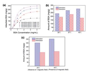
Fig. 8 (a) The influence of BSA initial concentration on BSA adsorption of IPN-pNIPAm@Fe $_2$ O $_3$ -SiO $_2$  nanogels, (b) the influence of temperature on BSA adsorption and desorption of IPN-pNIPAm@Fe $_2$ O $_3$ -SiO $_2$  nanogels, and (c) the influence of applied magnetic field on BSA adsorption of IPN-pNIPAm@Fe $_2$ O $_3$ -SiO $_2$  nanogels.
