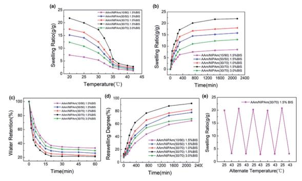
Fig. 7 Swelling behavior of the IPN-pNIPAm@Fe<sub>2</sub>O<sub>3</sub>-SiO<sub>2</sub> nanogels: (a) equilibrium swelling ratio of all nanogels at 20-45 °C; (b) equilibrium swelling ratio of all nanogels at 25 °C; (c) deswelling behavior of all nanogels at 40 °C; (d) reswelling behavior of all nanogels at 25 °C, and (e) reversible swelling/deswelling curve of the IPN-pNIPAm@Fe<sub>2</sub>O<sub>3</sub>-SiO<sub>2</sub> nanogels.
