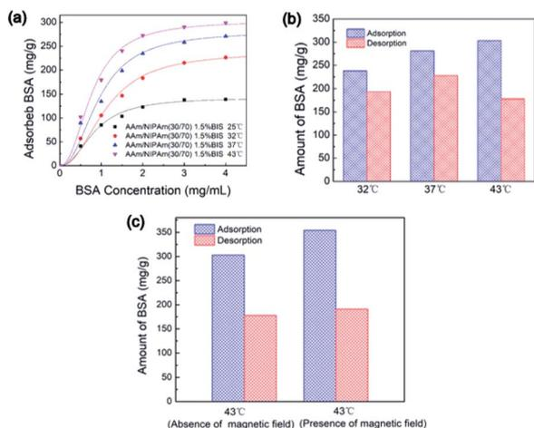
**Fig. 8** (a) The influence of BSA initial concentration on BSA adsorption of IPN-pNIPAm@Fe<sub>2</sub>O<sub>3</sub>-SiO<sub>2</sub> nanogels, (b) the influence of temperature on BSA adsorption and desorption of IPN-pNIPAm@Fe<sub>2</sub>O<sub>3</sub>-SiO<sub>2</sub> nanogels, and (c) the influence of applied magnetic field on BSA adsorption of IPN-pNIPAm@Fe<sub>2</sub>O<sub>3</sub>-SiO<sub>2</sub> nanogels.
