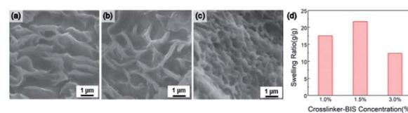
Fig. 6 SEM images of IPN-pNIPAm@Fe<sub>2</sub>O<sub>3</sub>-SiO<sub>2</sub> nanogels with different BIS crosslinker concentration: (a) AAm/NIPAm (30/70)-1.0%BIS, (b) AAm/NIPAm (30/70)-1.5%BIS, (c) AAm/NIPAm (30/70)-3.0%BIS, and (d) the effect of BIS crosslinker concentration on the swelling property of IPN-pNIPAm@Fe<sub>2</sub>O<sub>3</sub>-SiO<sub>2</sub> nanogels.
