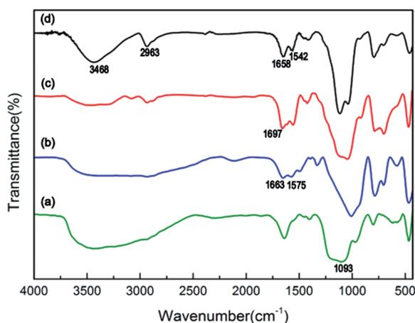
Fig. 4 FTIR spectrum of (a) Fe<sub>2</sub>O<sub>3</sub>-SiO<sub>2</sub> magnetic nanoparticles, (b) APTES-Fe<sub>2</sub>O<sub>3</sub>-SiO<sub>2</sub> magnetic nanoparticles, (c) AAm-Fe<sub>2</sub>O<sub>3</sub>-SiO<sub>2</sub> magnetic nanoparticles, and (d) IPN-pNIPAm@Fe<sub>2</sub>O<sub>3</sub>-SiO<sub>2</sub> nanogels.
