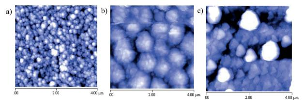
Fig. 4 Selected AFM images of (a) CsSnBr $_3$ , (b) CsSn $_2$ Br $_5$ , and (c) Cs $_2$ SnBr $_6$  on 4  $\mu m \times$  4  $\mu m$  area.
