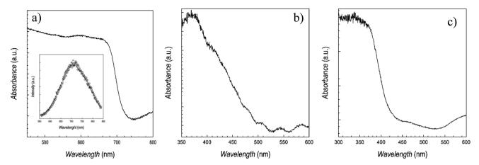
Fig. 3 UV-vis absorption spectra of (a) CsSnBr<sub>3</sub>, (b) CsSn<sub>2</sub>Br<sub>5</sub>, and (c) Cs<sub>2</sub>SnBr<sub>6</sub>. Inset of panel (a) reports the photoluminescence spectrum of CsSnBr<sub>3</sub>.
