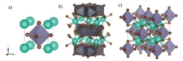
Fig. 1 Sketch of the crystal structures of (a)  $CsSnBr_3$ , (b)  $CsSn_2Br_5$ , and (c)  $Cs_2SnBr_6$  showing the peculiar octahedra arrangement in the different structures (see main text for details).
