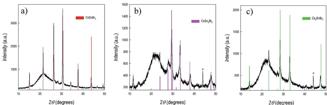
Fig. 2 X-ray diffraction patterns of (a)  $\text{CsSnBr}_3$ , (b)  $\text{CsSn}_2\text{Br}_5$ , and (c)  $\text{Cs}_2\text{SnBr}_6$ . Vertical red bars refer to the calculated pattern for each phase. Asterisk indicates reflection from the sample holder.
