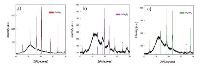
Fig. 2 X-ray diffraction patterns of (a)  $CsSnBr_5$ , (b)  $CsSn_2Br_5$ , and (c)  $Cs_2SnBr_6$ . Vertical red bars refer to the calculated pattern for each phase. Asterisk indicates reflection from the sample holder.
