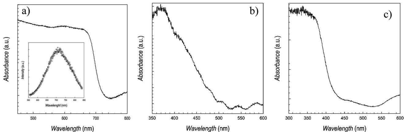
Fig. 3 UV-vis absorption spectra of (a)  $\text{CsSnBr}_3$ , (b)  $\text{CsSn}_2\text{Br}_5$ , and (c)  $\text{Cs}_2\text{SnBr}_6$ . Inset of panel (a) reports the photoluminescence spectrum of  $\text{CsSnBr}_3$ .
