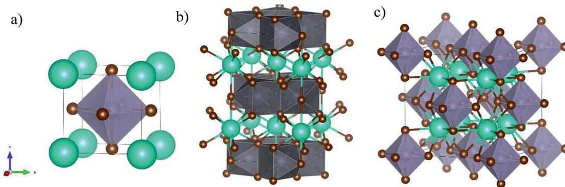
Fig. 1 Sketch of the crystal structures of (a)  $\text{CsSnBr}_3$ , (b)  $\text{CsSn}_2\text{Br}_5$ , and (c)  $\text{Cs}_2\text{SnBr}_6$  showing the peculiar octahedra arrangement in the different structures (see main text for details).
