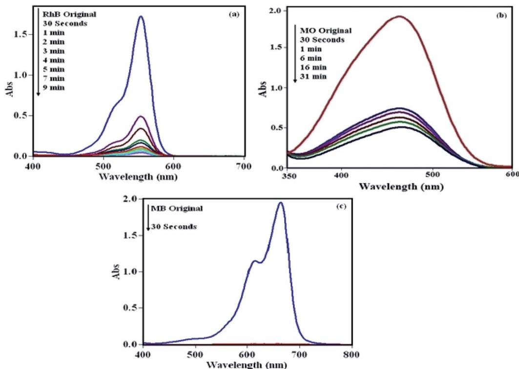
Fig. 4 UV-vis spectra of the adsorption of three dyes over POM/CFO/MIL-101(Cr): (a) RhB, (b) MO, and (c) MB. Adsorbent dosage = 30 mg, [dye]<sub>0</sub> = 25 mg L<sup>-1</sup>, 30 mL, temp = 25 °C.
