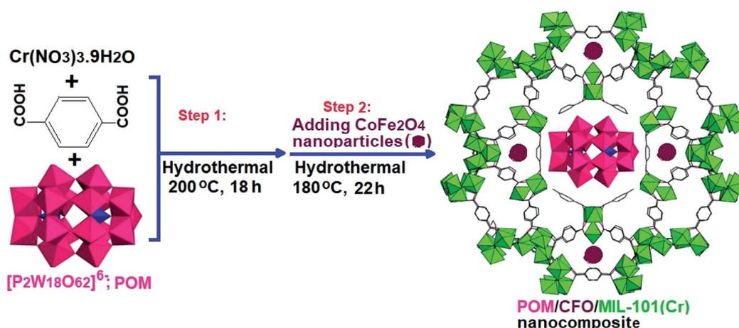
Scheme 1 The preparation process of the POM/CFO/MIL-101(Cr) nanocomposite.
