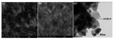
Fig. 5 (a and b) SEM micrographs at two different magnifications and (c) TEM image of PdO-2Mn<sub>2</sub>O<sub>3</sub>.
