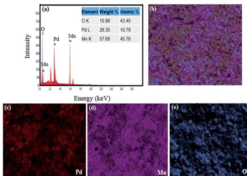
Fig. 3 (a) Elemental analysis of phyto-fabricated PdO–2Mn<sub>2</sub>O<sub>3</sub> and (b)–(e) elemental mapping images of individual O, Mn, and Pd.
