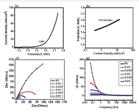
Fig. 7 Electro-catalytic measurements towards OER: (a) polarization curves, (b) Tafel slopes, (c) Nyquist plot at various potentials, (d) Bode plot showing variation in impedance as a function of frequency.
