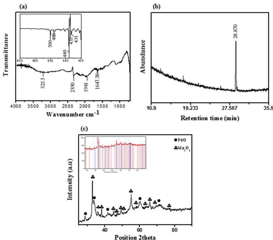
Fig. 2 (a) FTIR spectrum, (b) GCMS chromatogram and (c) X-ray diffractogram of synthesized PdO–2Mn<sub>2</sub>O<sub>3</sub>.
