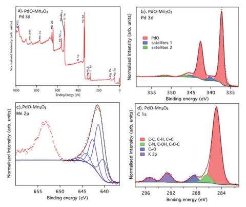
Fig. 4 XPS spectra recorded from PdO- $2Mn_2O_3$ : (a) survey spectra, (b) Pd 3d, (c) Mn 2p, (d) C 1s core levels.
