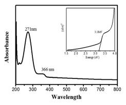
Fig. 6 Optical analysis of PdO-2Mn<sub>2</sub>O<sub>3</sub> by UV-vis absorption spectra.
