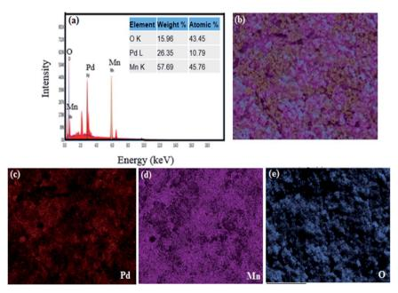
Fig. 3 (a) Elemental analysis of phyto-fabricated  $PdO-2Mn_2O_3$  and (b)–(e) elemental mapping images of individual O, Mn, and Pd.
