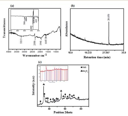
Fig. 2 (a) FTIR spectrum, (b) GCMS chromatogram and (c) X-ray diffractogram of synthesized PdO-2Mn<sub>2</sub>O<sub>3</sub>.
