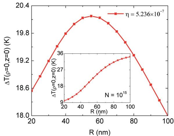
Fig. 5 The maximum temperature of  $\Delta T$  of the floating PANi-cotton fabric as a function of nanoparticle radius when the volume fraction  $\eta = 5.236 \times 10^{-7}$  is fixed. The inset shows the same functional dependence at a fixed nanoparticle density  $N = 10^{15}$  particles per  $\text{m}^3$  (inset).
