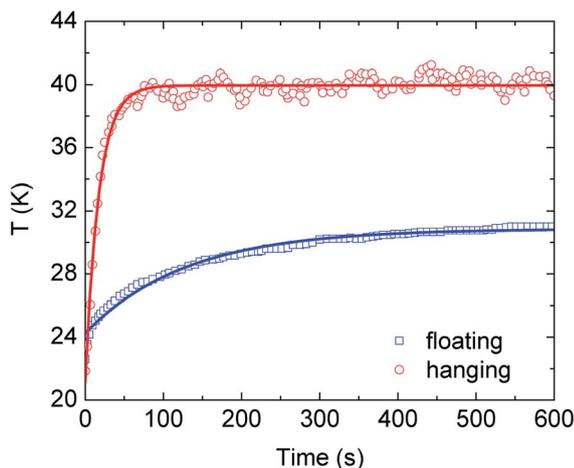
Fig. 2 Experimental<sup>9</sup> and theoretical (eqn (8)) temperature at the surface ( $z = 0$ ) of the hanging and floating PANi-cotton membrane as a function of time under sunlight irradiation. Discrete data points and solid curves correspond to the experimental data and theoretical calculations, respectively.
