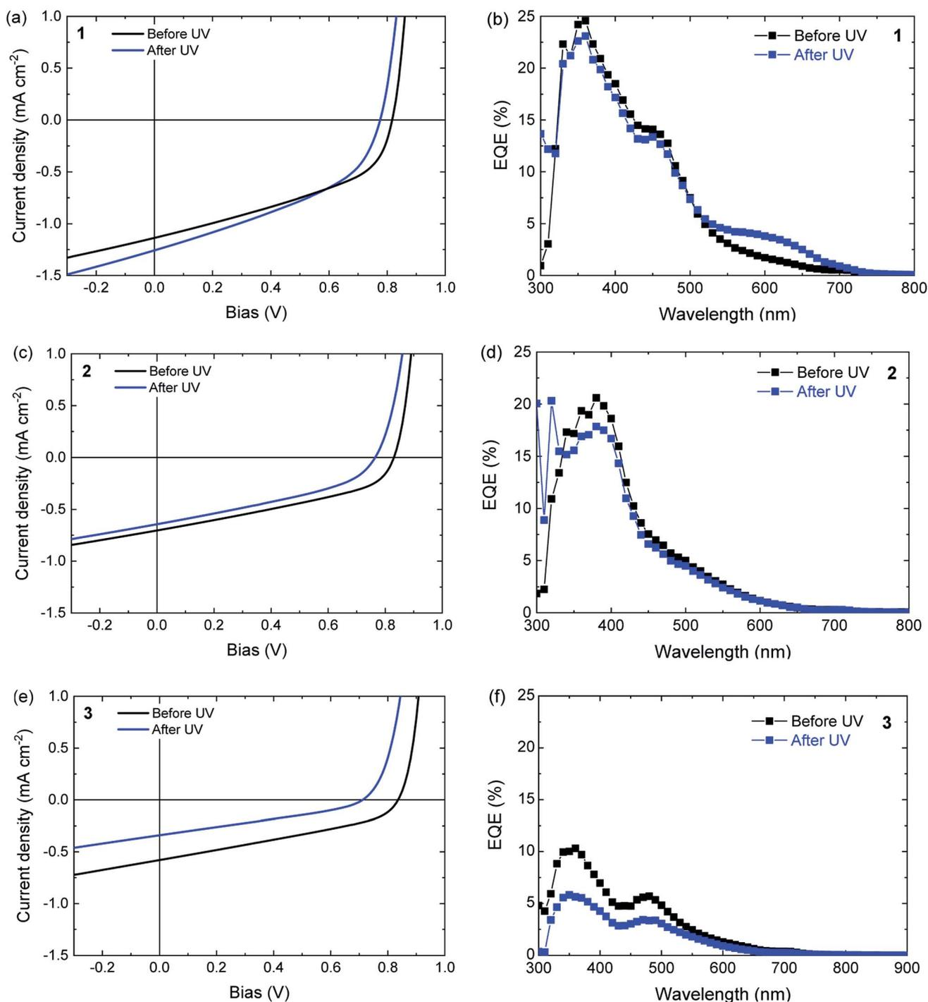
Fig. 6 (a, c and e) Current density–voltage ( $J$ – $V$ ) characteristics of ternary DAE/poly-TPD/PC<sub>61</sub>BM solar cells before and after UV illumination to convert the ring-open isomer to the ring-closed isomer, measured under simulated AM1.5 G solar light. (b, d and f) Corresponding EQE spectra. (a and b) For DAE **1**, (c and d) for DAE **2**, (e and f) for DAE **3**.
