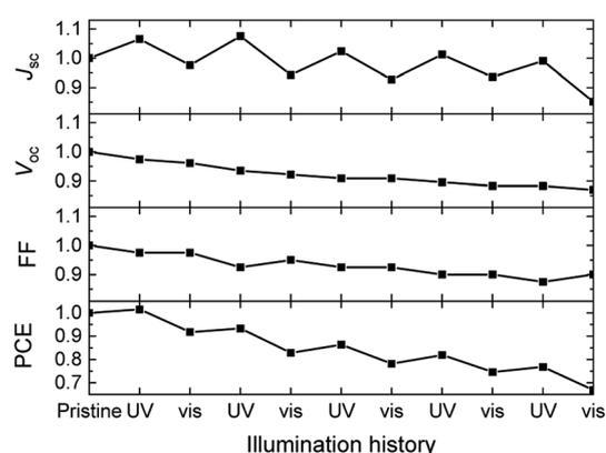
Fig. 7 Evolution of the normalized photovoltaic parameters of solar cells based on **1**/poly-TPD/PC<sub>61</sub>BM blends in five cycles of 30 min of UV illumination followed by 30 min exposure to visible light.
