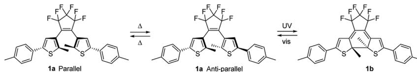
Fig. 3 The parallel and antiparallel conformations of **1a** that are interswitchable in solution but are less likely to interconvert in the solid phase. Correspondingly in the solid state the photochromic ring closure to **1b** will occur from the antiparallel conformation of **1a**.
