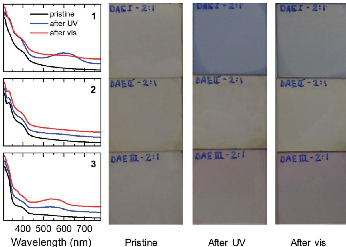
Fig. 5 UV-vis absorption spectra and photographs of ternary blends of 1–3, PC<sub>61</sub>BM, and poly-TPD. The ratio DAE/poly-TPD/PC<sub>61</sub>BM weight ratio was 10 : 1 : 4. The samples were consecutively measured as pristine samples, after UV illumination, and after illumination with visible light as detailed in the Experimental section. The UV-vis spectra are offset vertically for clarity.
