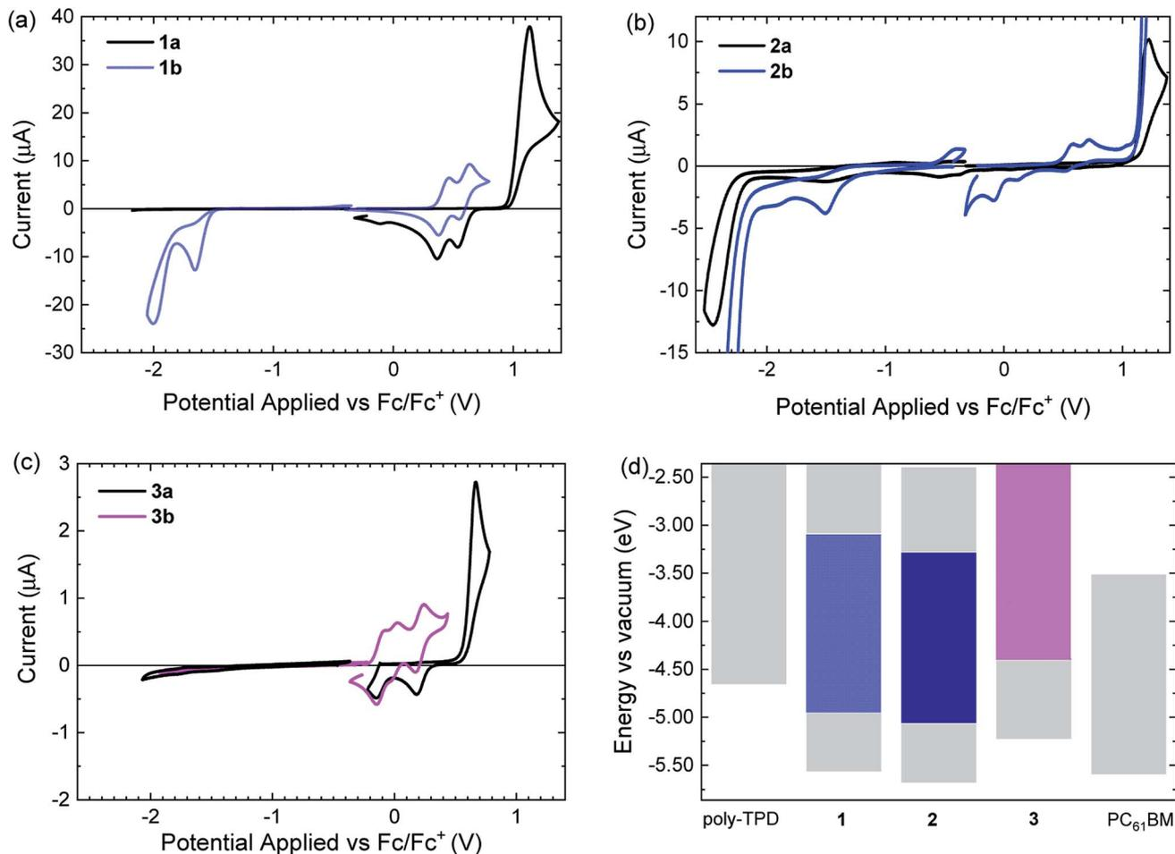
Fig. 4 (a–c) Cyclic voltammograms of open-ring (black solid lines) and closed-ring isomers (colored solid lines) of 1–3 in acetonitrile. Potentials are versus Fc/Fc<sup>+</sup>. (d) Comparison of energy levels of 1–3 with those of poly-TPD and PC<sub>61</sub>BM.
