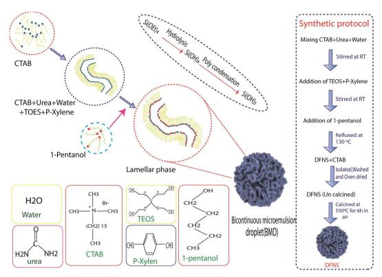
Fig. 1 Graphic illustration of DFNS synthesis.
