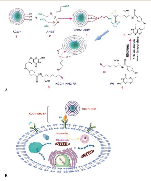
Fig. 7 (A) Schematic representation of the functionalization of KCC-1-NH<sub>2</sub>. (B) Schematic illustration of the mechanism of the developed FR-positive cytosensor.<sup>121</sup>
