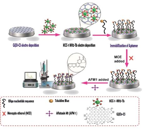
Fig. 8 The aptasensor assembly procedure and its application in the monitoring of AF M1.<sup>125</sup>
