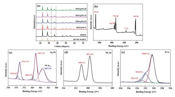
Fig. 2 (a) XRD patterns of the HMNb, HMAgNb-5, HMAgNb-10, HMAgNb-15, HMAgNb-20 and standard XRD pattern of Nb<sub>2</sub>O<sub>5</sub> (JCPDS no. 30-0873). (b) XPS survey of the HMAgNb-15. (c-e) High-resolution XPS spectra for the Ag 3d, Nb 3d, and O 1s.
