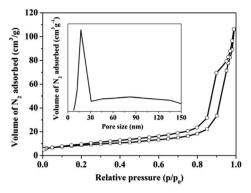
Fig. 5  $N_2$  adsorption and desorption isotherms of the HMAgNb-15, illustrated with pore size distribution curve.
