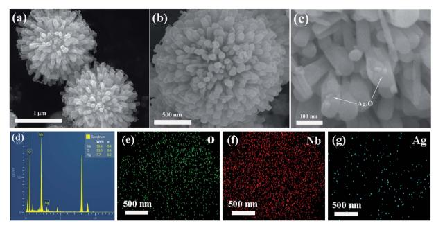
Fig. 3 (a) SEM image of HMNb. (b) SEM and (c) HRSEM images of HMAqNb-15 and (d-g) its corresponding EDS pattern and elemental mapping images of O, Nb, Ag.
