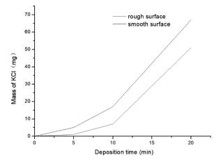
Fig. 7 KCl condensation on surfaces of different roughness.
