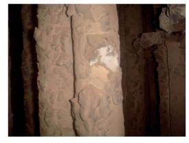
Fig. 2 Deposits on high temperature superheater.
