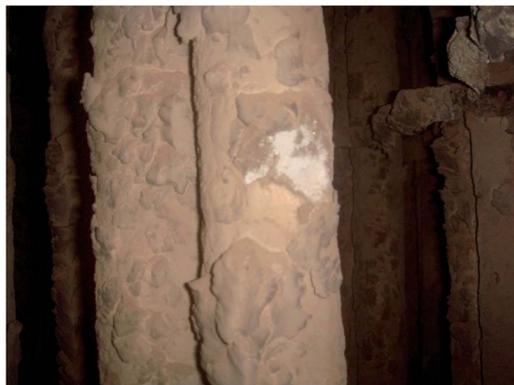
Fig. 2 Deposits on high temperature superheater.
