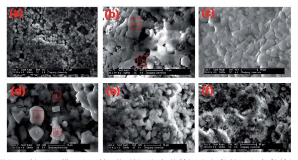
Fig. 5 SEM pictures of deposits at different times of deposition. (a) deposits after 1 h, (b) deposits after 2 h, (c) deposits after 5 h, (d) deposits after 1 h, (e) deposits after 1 day, (f) deposits after 2 days.
