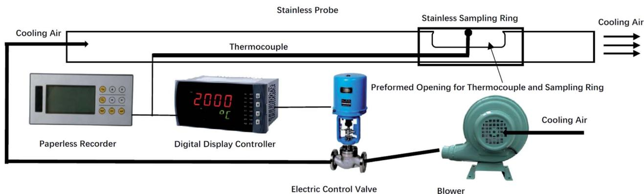
Fig. 4 Ash deposit probe with temperature control.
