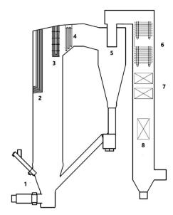
Fig. 1 The 50 MW CFB boiler: (1) feeder; (2) water wall; (3) platen superheater; (4) high-temperature superheater; (5) cyclone separator; (6) low-temperature superheater; (7) economizer; (8) air preheater.
