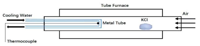
Fig. 6 KCl condensation experiment system.
