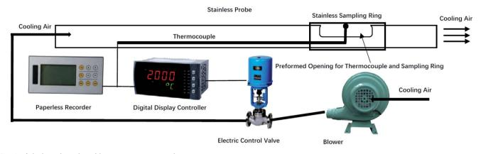
Fig. 4 Ash deposit probe with temperature control.
