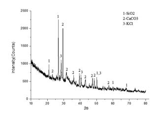
Fig. 3 XRD result of the fly ash.
