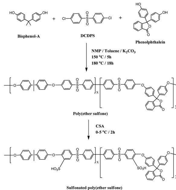
Scheme 1 Schematic for the synthesis of sulfonated poly(ether sulfone).
