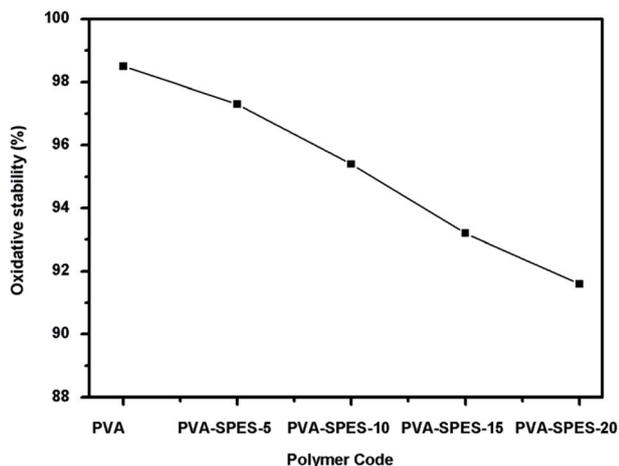
Fig. 5 Oxidative stability of the PVA and PVA-SPES blend membranes.
