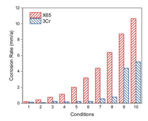
Fig. 7 Corrosion rate of carbon steel and 3Cr steel measured under different conditions in Table 4.
