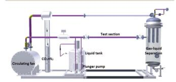
Fig. 2 Schematic of the flow loop tests.
