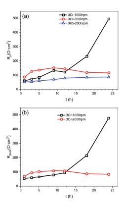
Fig. 5 The  $R_{\text{pore}}$  value (a) and  $R_{\text{p}}$  value (b) obtained from the EIS results.
