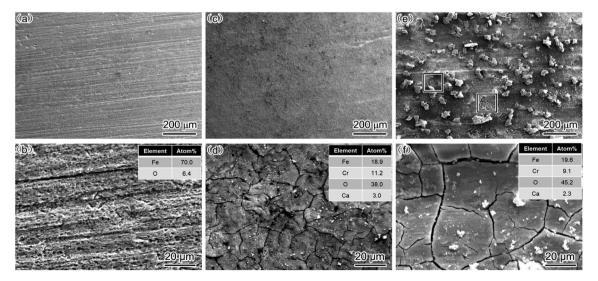
Fig. 6 SEM-SE image and EDS analysis of corrosion scale (a and b) carbon steel, 2000 rpm; (c and d) 3Cr steel, 1000 rpm; (e and f) 3Cr steel, 2000 rpm.
