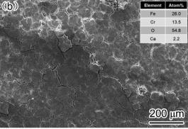
Fig. 9 SEM-SE image of corrosion film on (a) carbon steel and (b) 3Cr steel after flow loop tests under condition 6 in Table 4.
