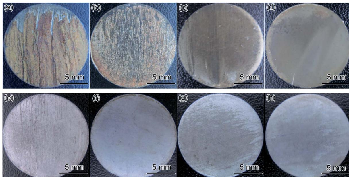
Fig. 8 Macro morphologies of coupons with (a–d) and without (e–h) the corrosion film after flow loop tests under conditions 5 and 6 in Table 4: (a and e) carbon steel, 24 h; (b and f) carbon steel, 72 h; (c and g) 3Cr steel, 24 h; (d and h) 3Cr steel, 72 h.
