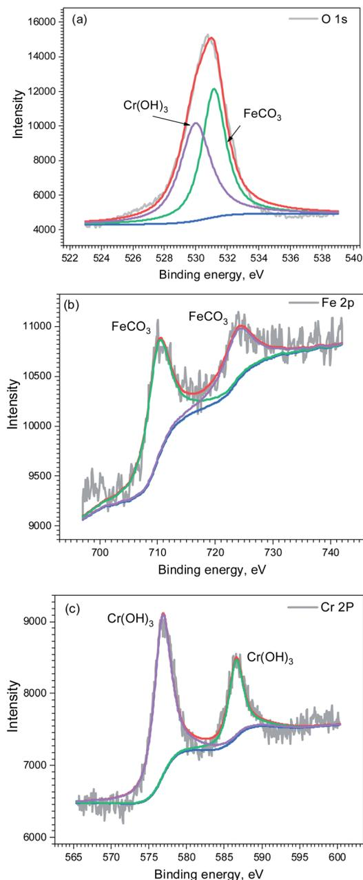
Fig. 10 XPS analysis of corrosion scale formed on 3Cr steel surface after flow loop tests under condition 6 in Table 4: (a) O 1s; (b) Fe 2p<sub>2/3</sub>; (c) Cr 2p<sub>2/3</sub>.
