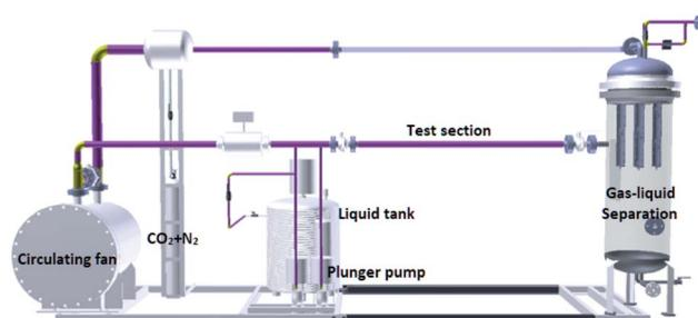
Fig. 2 Schematic of the flow loop tests.
