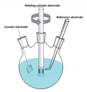
Fig. 1 Schematic of the rotating cylinder electrode tests.
