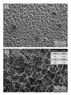
Fig. 11 SEM-SE image of corrosion film on 3Cr steel after flow loop tests under condition 10 in Table 4. (a) Carbon steel, (b) 3Cr steel.
