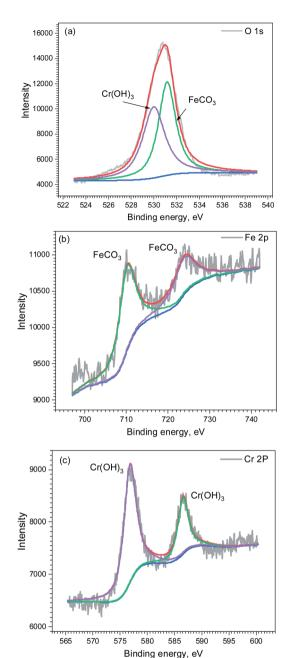
Fig. 10 XPS analysis of corrosion scale formed on 3Cr steel surface after flow loop tests under condition 6 in Table 4: (a) O 1s; (b) Fe  $2p_{2/3}$ ; (c) Cr  $2p_{2/3}$ .
