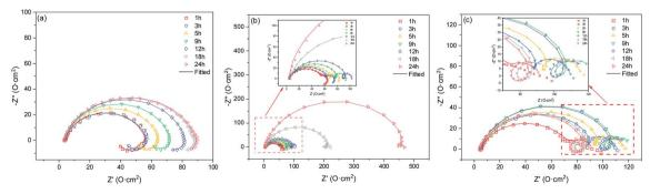
Fig. 3 Nyquist diagrams (a) carbon steel, 2000 rpm; (b) 3Cr steel, 1000 rpm; (c) 3Cr steel, 2000 rpm.
