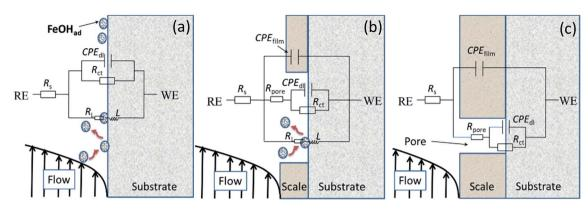
Fig. 4 Equivalent circuits used for modeling the EIS results in Fig. 3.
