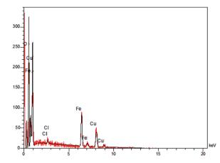
Fig. 6 EDX patterns of nano-Fe<sub>3</sub>O<sub>4</sub>@walnut shell/Cu(II)
