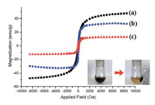
Fig. 4 Magnetization loops of (a)  $Fe_3O_4$  (b) nano- $Fe_3O_4$ @walnut shell, (c) nano- $Fe_3O_4$ @walnut shell/Cu( $\iota$ ).
