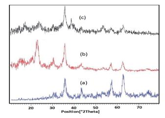
Fig. 2 XRD patterns of the (a)  $Fe_3O_4$  (b) nano- $Fe_3O_4$ @walnut shell, (c) nano- $Fe_3O_4$ @walnut shell/Cu( $\shortparallel$ ).
