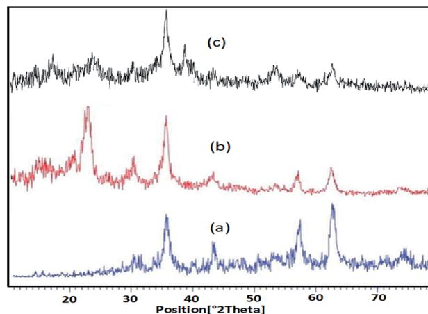
Fig. 2 XRD patterns of the (a) Fe<sub>3</sub>O<sub>4</sub> (b) nano-Fe<sub>3</sub>O<sub>4</sub>@walnut shell, (c) nano-Fe<sub>3</sub>O<sub>4</sub>@walnut shell/Cu(II).
