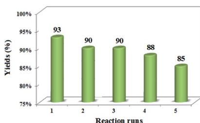
Fig. 7 Reusability of catalyst in the reaction between formaldehyde, aniline, and β-naphthol.
