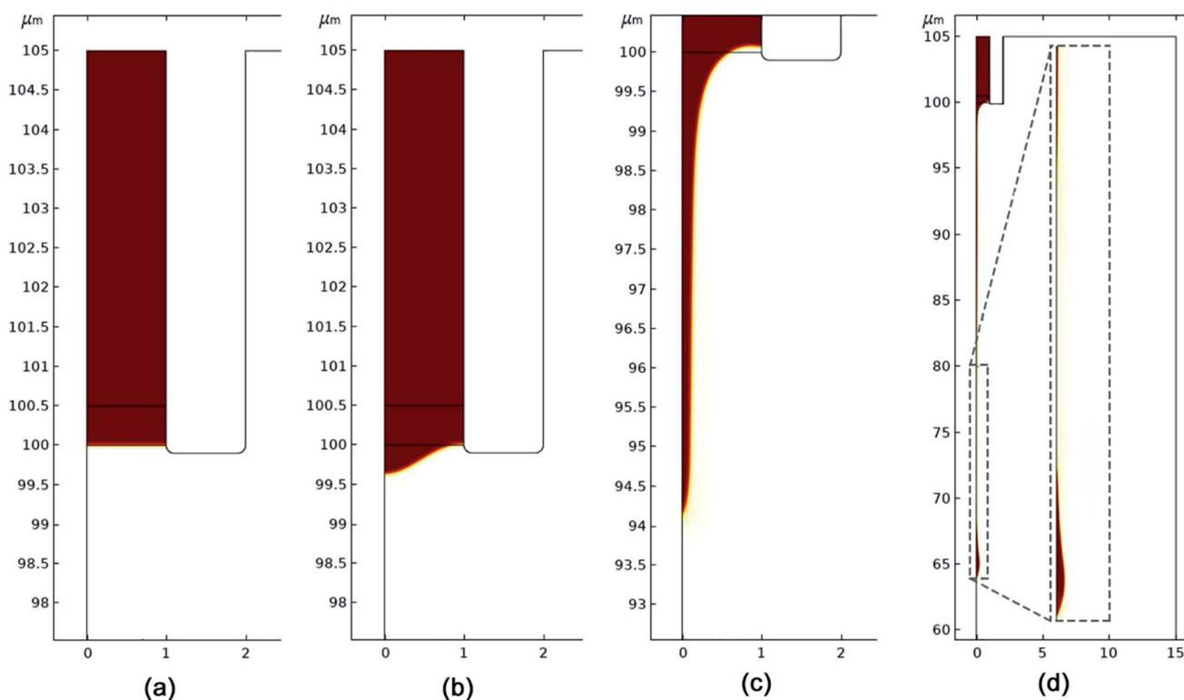
Fig. 3 Simulated octanol cone-jet from a 2  $\mu\text{m}$  nozzle for flow rate of  $1 \times 10^{-12} \text{ m}^3 \text{ s}^{-1}$  using the COMSOL electrohydrodynamic model at different time instants: (a) 0 s, (b)  $4 \times 10^{-7}$  s, (c)  $6 \times 10^{-7}$  s and (d)  $1.7 \times 10^{-6}$  s. The capability of the phase-field model in predicting droplet breakup is established in panel 'd'.
