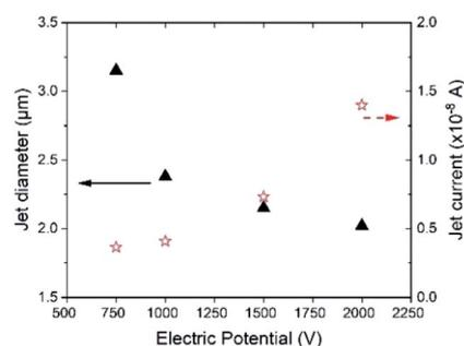
Fig. 5 The impact of voltage on the resultant jet diameter and current in the case of tetradecane. Here,  $Q_{\text{in}} = 5 \times 10^{-11} \text{m}^3 \text{s}^{-1}$  and  $D_{\text{nozzle}} = 10 \mu\text{m}$ .
