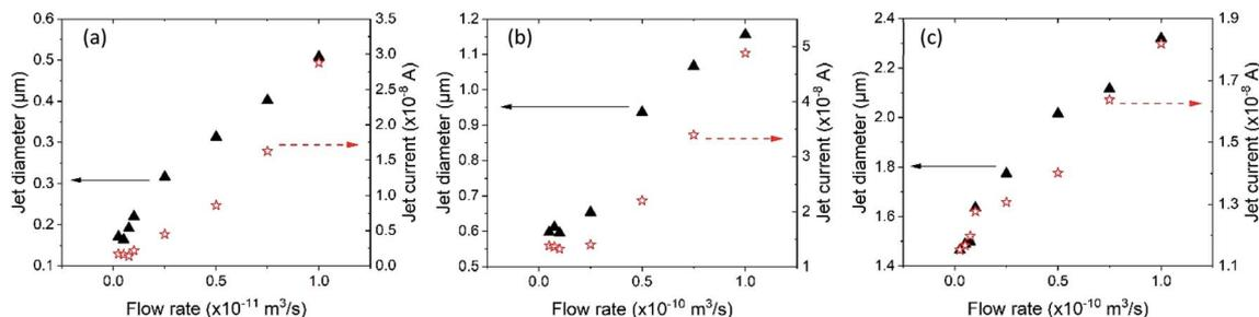
Fig. 4 Calculated jet diameter and current for different simulation cases: (a) octanol &  $D_{\text{nozzle}} = 2 \mu\text{m}$ ; (b) octanol &  $D_{\text{nozzle}} = 10 \mu\text{m}$ ; (c) tetradecane &  $D_{\text{nozzle}} = 10 \mu\text{m}$ .
