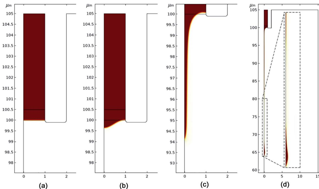
Fig. 3 Simulated octanol cone-jet from a 2  $\mu\text{m}$  nozzle for flow rate of  $1 \times 10^{-12} \text{ m}^3 \text{ s}^{-1}$  using the COMSOL electrohydrodynamic model at different time instants: (a) 0 s, (b)  $4 \times 10^{-7}$  s, (c)  $6 \times 10^{-7}$  s and (d)  $1.7 \times 10^{-6}$  s. The capability of the phase-field model in predicting droplet breakup is established in panel 'd'.
