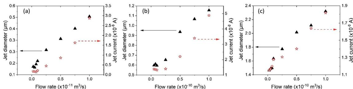
Fig. 4 Calculated jet diameter and current for different simulation cases: (a) octanol &  $D_{\text{nozzle}} = 2 \mu\text{m}$ ; (b) octanol &  $D_{\text{nozzle}} = 10 \mu\text{m}$ ; (c) tetradecane &  $D_{\text{nozzle}} = 10 \mu\text{m}$ .
