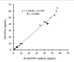
Fig. 6 Correlation analysis between the Cobas E601 chemiluminescence immunoassay analyzer and the proposed NS-LFIA in quantifying AFP from 40 clinical serum samples.
