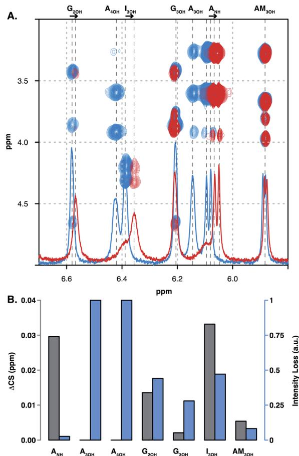
Fig. 7 Low temperature NMR of the carbohydrate amine and hydroxyl groups. (A) Overlay of TOCSY and 1D- $^1\text{H}$  spectra of OXT alone (blue) and in complex with FP (red). Assignments of hydroxyl residues of FP appear on the bottom. Arrows indicate system shifts. (B)  $\Delta\text{CS}$  of hydroxyl residues of FP in the F2 dimension (grey bars) and normalised signal intensity loss (blue bars; 0 = no intensity change and 1 = the signal has completely disappeared).
