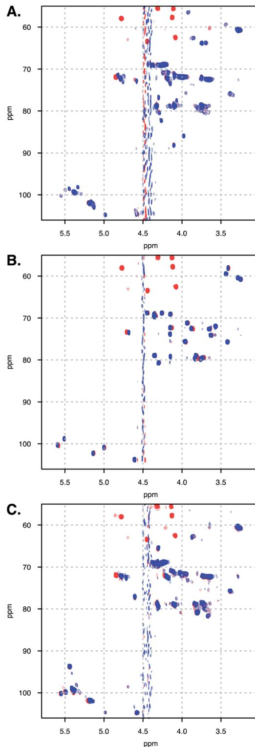
Fig. 5 Spectra overlay of free (A) **DAL**, (B) **FP** and (C) **DP6** (blue), and in complex with **OXT** (red). Spectra measured at 328 K.
