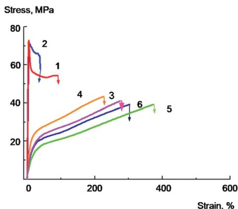
Fig. 8 Stress–strain curves for the dampened films: PVA (1), PVA/GO containing 2 wt% of GO (2), PVA/Gly containing 10 wt% of glycerol (3), PVA/GO/Gly containing 2 wt% of GO and 10 wt% of glycerol (4), PVA/Gly containing 20 wt% of glycerol (5), PVA/GO/Gly containing 2 wt% of GO and 20 wt% of glycerol (6).
