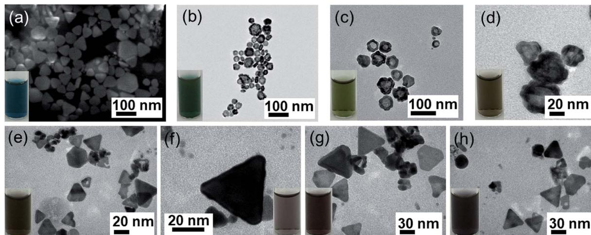
Fig. 2 (a) SEM image of Ag NPI4 used as template seeds. The typical TEM images of (b) Ag–Au1 ( $x = 0.1 \mu\text{mol}$ ), (c) Ag–Au2 ( $x = 0.2 \mu\text{mol}$ ), (d) Ag–Au3 ( $x = 0.4 \mu\text{mol}$ ), (e) Ag–Au4 ( $x = 0.6 \mu\text{mol}$ ), (f) Ag–Au6 ( $x = 1.0 \mu\text{mol}$ ), (g) Ag–Au9 ( $x = 2.0 \mu\text{mol}$ ) and (h) Ag–Au12 ( $x = 3.4 \mu\text{mol}$ ). Insets in each image are photographs of the corresponding bimetallic Ag–Au core/shell or alloy solutions.
