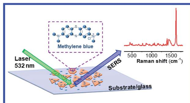
Fig. 10 Schematic illustration of SERS measurement principle.
