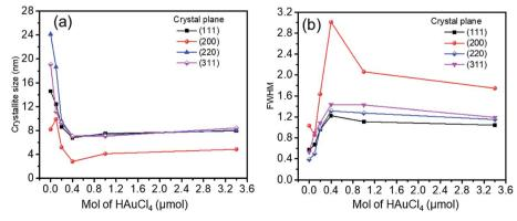
Fig. 5 (a) Crystalline size, and (b) FWHM as a function of HAuCl<sub>4</sub> amount at all crystal facets (111), (200), (220) and (311).
