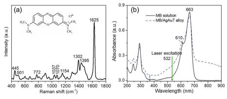
Fig. 9 (a) Raman spectra of only MB  $(10^{-4} \text{ M})$  and chemical structure (inset). (b) Absorption spectra of pure MB and the mixture of MB and Ag-Au alloy nanoplates.
