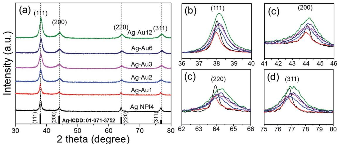
Fig. 4 (a) XRD analysis of the silver nanoplate (Ag NPL4) and bimetallic Ag–Au nanoplates (Ag–Au1, Ag–Au2, Ag–Au3, Ag–Au6, and Ag–Au12) (b–d) the diffraction peaks at around  $37.9^\circ$  (111),  $44.07^\circ$  (200),  $63.9^\circ$  (220), and  $76.7^\circ$  (311).
