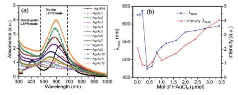
Fig. 3 (a) UV-Vis spectra of Ag NPl4 and Ag-Au samples with different amounts of HAuCl<sub>4</sub>. (b) The dependence of maximum wavelength of LSPRs (blue line) and maximum intensity (red line) of dipolar LSPR mode as a function of concentration of HAuCla.
