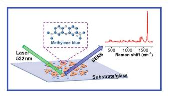
Fig. 10 Schematic illustration of SERS measurement principle.
