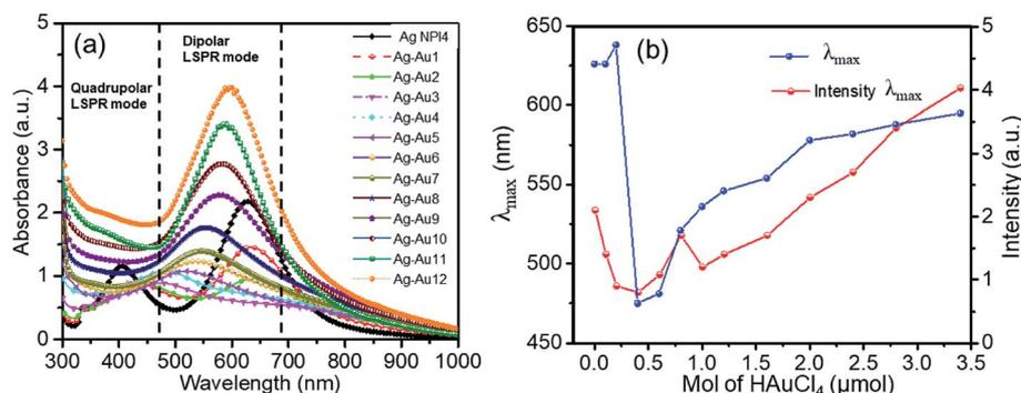
Fig. 3 (a) UV-Vis spectra of Ag NPI4 and Ag–Au samples with different amounts of  $\text{HAuCl}_4$ . (b) The dependence of maximum wavelength of LSPRs (blue line) and maximum intensity (red line) of dipolar LSPR mode as a function of concentration of  $\text{HAuCl}_4$ .
