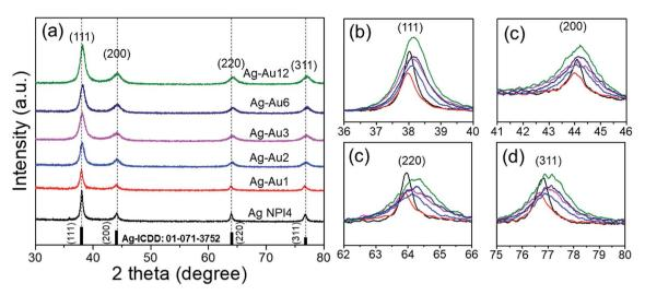
Fig. 4 (a) XRD analysis of the silver nanoplate (Ag NPl4) and bimetallic Ag–Au nanoplates (Ag–Au1, Ag–Au2, Ag–Au3, Ag–Au6, and Ag–Au12) (b-d) the diffraction peaks at around 37.9° (111), 44.07° (200), 63.9° (220), and 76.7° (311).
