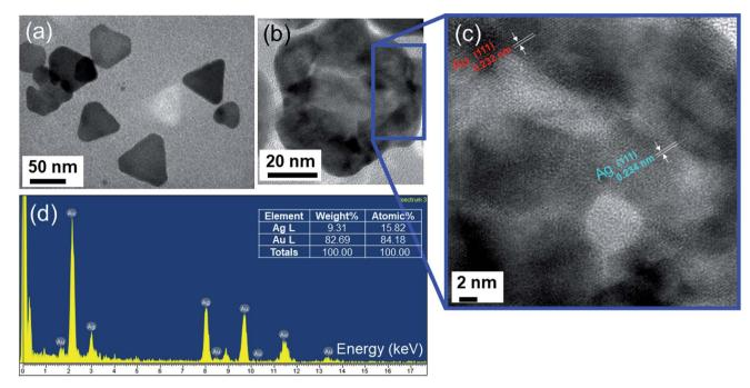
Fig. 7 (a) Low-resolution TEM image of Ag-Au alloy nanoplate. (b) HRTEM of a typical synthesized single Ag-Au alloy and (c) HRTEM image of a part of this alloy, which indicated the lattice plane constants of Ag (0.234 nm) and Au (0.232 nm). (d) EDS spectrum of (b) which shows the contribution of Ag and Au atoms in the Ag-Au alloy ( $x = 3.4 \mu mol$ ).
