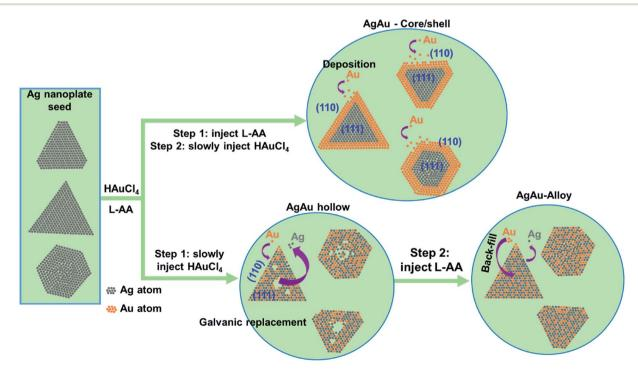
Fig. 8 Schematic illustration of the formation mechanism Aq-Au nanoplate core/shell and alloy.
