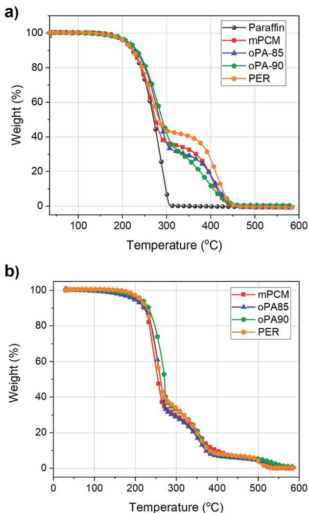
Fig. 2 TGA curves obtained under (a) N<sub>2</sub> gas flow (c) switch mode of N<sub>2</sub>/O<sub>2</sub> gas flow.
