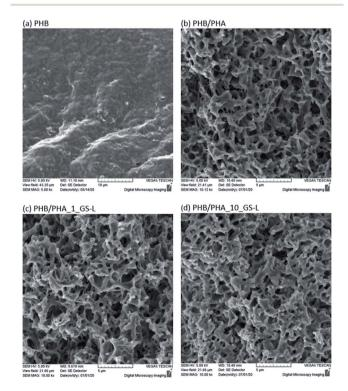
Fig. 8 SEM morphology of neat PHB, PHB/PHA, PHB/PHA\_1-GS-L and PHB/PHA\_10-GS-L.
