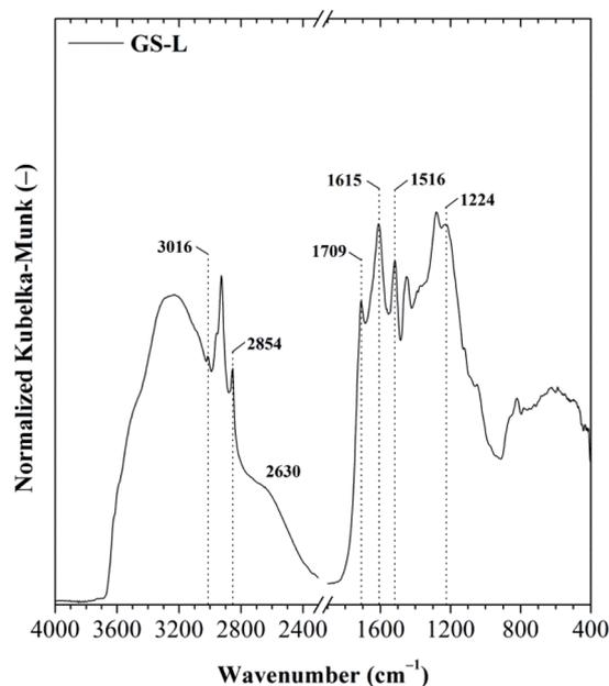
Fig. 3 ATR-IR spectrum of the grape seeds lignin (GS-L).
