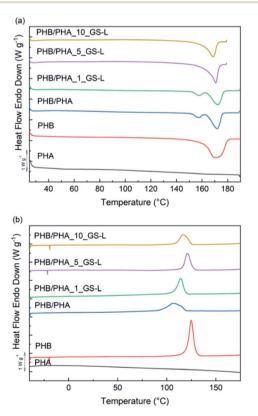
**Fig. 5** DSC (a) first heating scans and (b) cooling scans for PHA, PHB, PHB/PHA, PHB/PHA\_1\_GS-L, PHB/PHA\_5\_GS-L, and PHB/PHA\_10\_GS-L.
