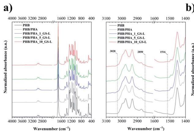
Fig. 4 ATR-FTIR spectra of neat PHB and PHB/PHA blends with or without grape seeds lignin (GS-L), (a) spectral range of  $4000\text{--}400\text{ cm}^{-1}$  and (b) spectral range of  $3100\text{--}1400\text{ cm}^{-1}$ .
