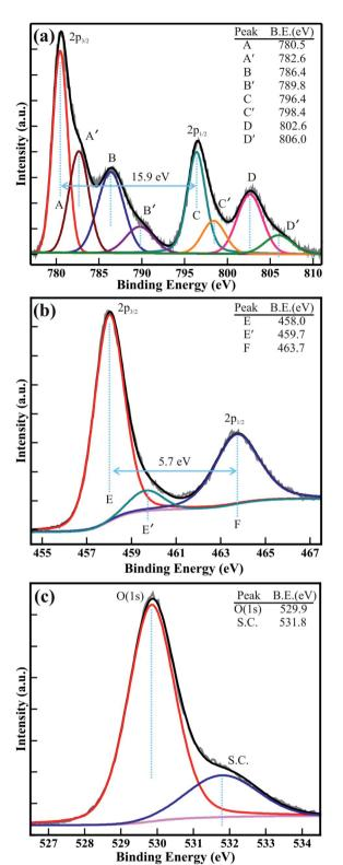
Fig. 6 Typical high-resolution XPS spectra of the (a) Co(2p), (b) Ti(2p), and (c) O(1s) core levels of the mesoporous CTO microrods.
