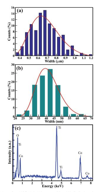
Fig. 4 (a and b) Statistical histogram of the width distribution microrods and nanoparticles, respectively, and (c) EDS spectra of mesoporous CTO microrods.
