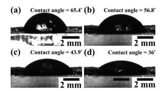
Fig. 7 Contact angle measurement showing the interface of the aqueous KOH electrolyte of (a) 0.5 M, (b) 1 M, (c) 1.5 M, and (d) 2 M concentration on the surface of the working electrode of mesoporous CTO microrods.
