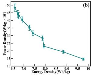
Fig. 10 (a) Nyquist (EIS) plot of the mesoporous CTO microrods obtained before and after cyclic stability studies. Inset shows the best fitted equivalent circuit model. (b) Evaluated specific energy and specific power of the mesoporous CTO microrods.
