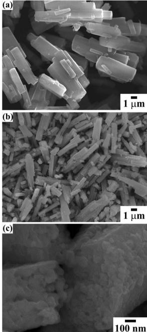
Fig. 3 FESEM image of (a) as-synthesized and (b) annealed  $CoTiO_3$  microrod. (c) The high-magnification FESEM image confirms the formation of mesoporous  $CoTiO_3$  microrod composed of hierarchically interlinked nanoparticles.
