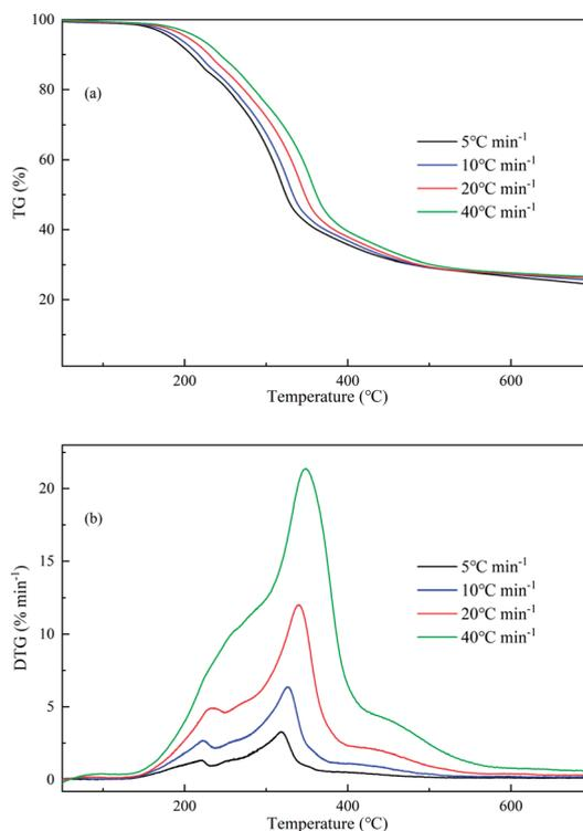
**Fig. 1** TG and DTG curves of SSR.
