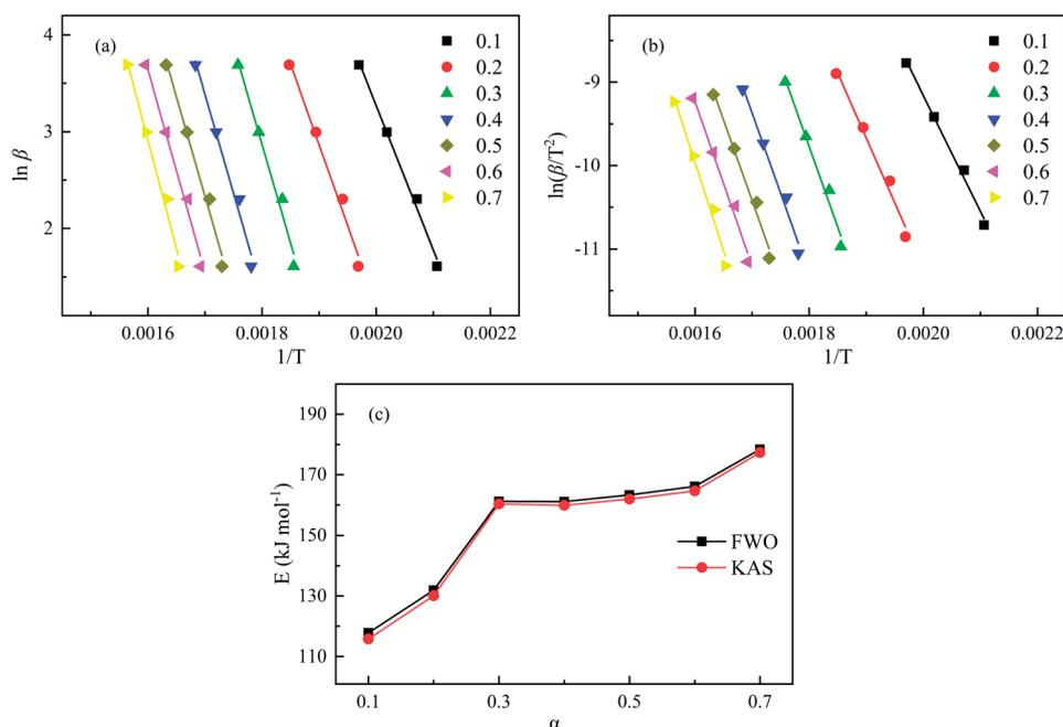
Fig. 2 Kinetic plots according to FWO (a) and KAS (b) and the corresponding activation energies (c) of SSR.
