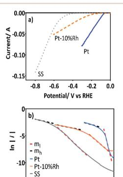
Fig. 3 (a) PC of the Pt (blue), Pt–10%Rh (orange) and SS (gray) cathodes for HER in 0.5 mol L $^{-1}$  H $_2$ SO $_4$  (LSV scan rate =5 mV s $^{-1}$ ). (b) The corresponding Tafel plots of Pt (blue), Pt–10%Rh (orange) and SS (gray) calculated from data of plots in (a). Dashed lines show the overpotential regions at which the Tafel slopes were calculated.
