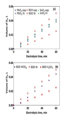
Fig. 6 The amount of the gas (in L) obtained by theoretical calculation (empty symbols) and by experimental measurements (full symbols) as a function of the time for: (a) 0.5 mol L $^{-1}$  H<sub>2</sub>SO<sub>4</sub> + 20 ppm MR and (b) 0.5 mol L $^{-1}$  H<sub>2</sub>SO<sub>4</sub> + 20 ppm MR (red symbol) and 0.5 M HClO<sub>4</sub> + 20 ppm MR (violet symbol) solutions at 30 mA cm $^{-2}$  and 298 K.
