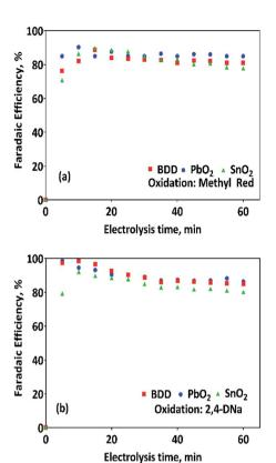
Fig. 5 Faradaic efficiencies (in %) calculated by using eqn (13) for (a) data of collected about the volume of hydrogen of Fig. 4a and (b) for that values of collected volume of hydrogen of Fig. 4b.
