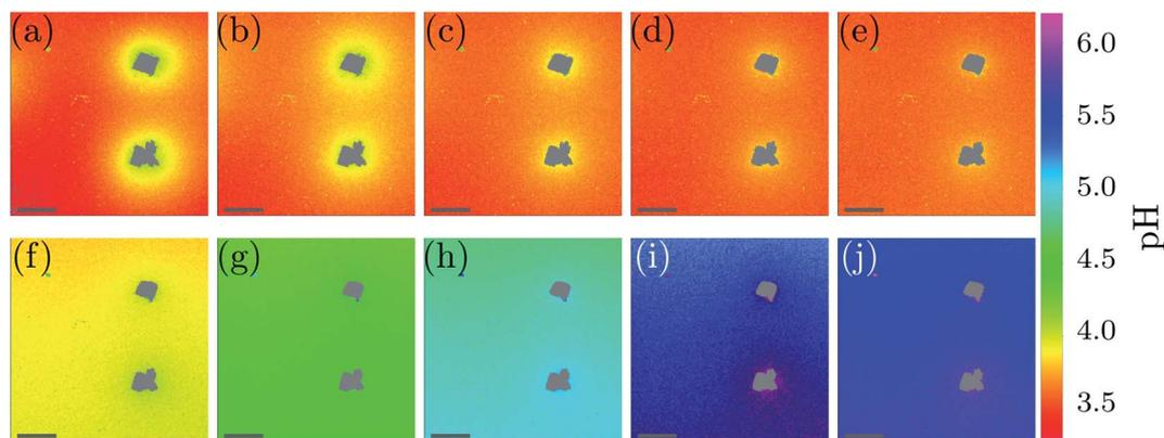
Fig. 4 Local pH monitoring of the dissolution: (a)–(e) shows time-points at the start of the measurement (=0 min), after 1 min, 2 min, 3 min and 5 min of the measurement. Also later time-points of the dissolution process are shown, *i.e.* (f) 10 min, (g) 15 min, (h) 20 min, (i) 25 min and (j) 30 min. The scale-bar is 75  $\mu\text{m}$ .
