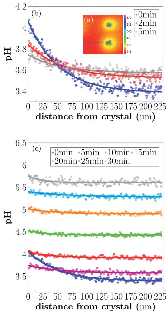
Fig. 5 pH profile close to a dissolving crystal for different time-points of dissolution. (a) Example image of local pH distribution during dissolution. Intensity profiles are extracted from the images along the dashed line. (b) Intensity profiles are given 0 min, 2 min, and 5 min of the reaction. (c) pH profiles for longer reaction times.
