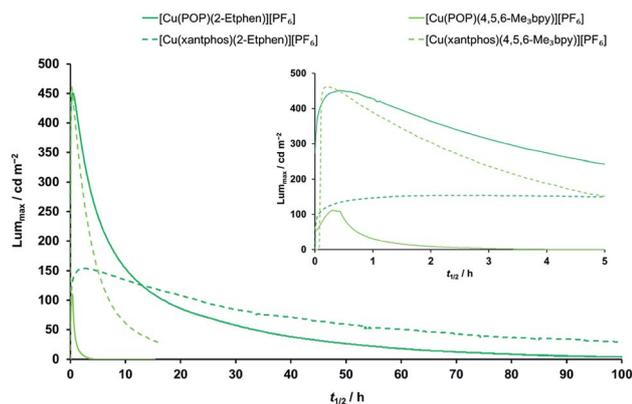
Fig. 10 Time evolution of luminance for ITO/PEDOT:PSS/[Cu(P<sup>P</sup>)(N<sup>N</sup>)]PF<sub>6</sub> : [Emim]PF<sub>6</sub> 4 : 1 molar ratio/Al LECs measured using a pulsed current driving and under continuous operation (average current density 100 A m<sup>-2</sup>). Inset shows the behaviour over the first five hours. For time evolution of further parameters (average voltage, power conversion efficiency, external quantum efficiency and electroluminescence spectra) see Fig. S38–S41.†
