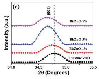
**Fig. 5** XRD analysis of (a) pristine ZnO NWs, (b) pristine and Bi-doped ZnO NWs for 1%, 3%, and 5% concentration, and (c) 002 peak for the pristine and Bi-doped ZnO NWs samples.
