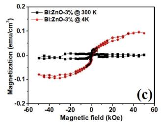
Fig. 10 SQUID plots at 300 K (close squares) and 4 K (closed circles) for (a) pristine ZnO, (b) Bi:ZnO-1%, and (c) Bi:ZnO-3% NWs.
