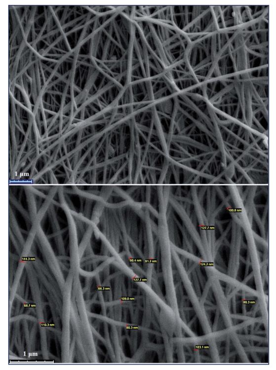
Fig. 4 SEM images and the distribution of the prepared nanofibers of electrospun PANI-b-PAA.
