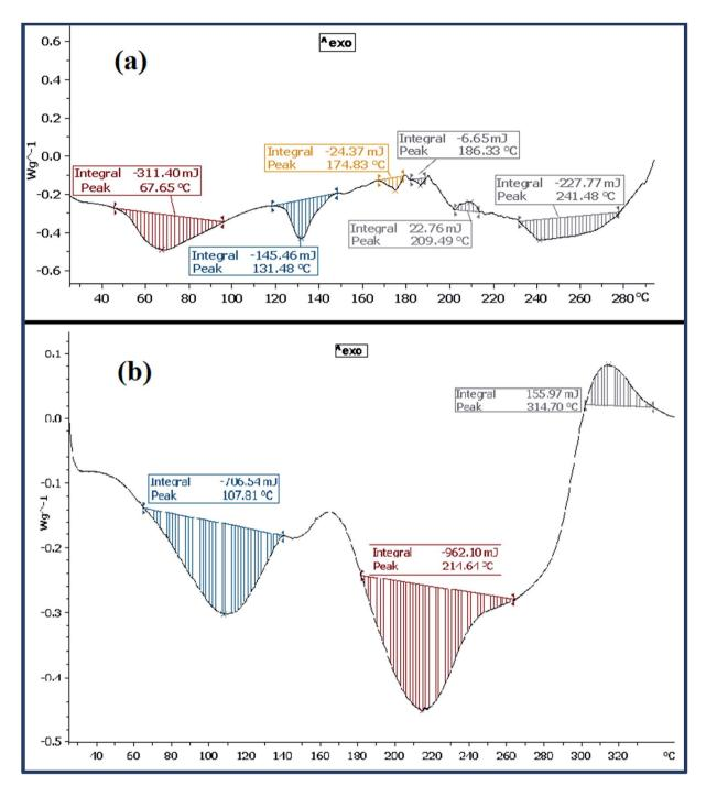
Fig. 7 DSC curves of CTA-PAA (a) and PANI-b-PAA (b).
