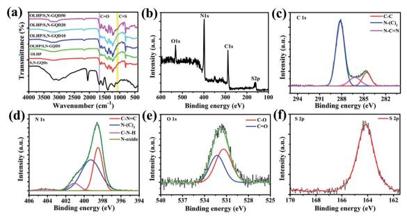
Fig. 3 (a) FTIR spectra of S,N-GQDs, OLHP and OLHP/S,N-GQDs, (b) XPS full scan, high resolution XPS of (c) C 1s, (d) N 1s, (e) O 1s and (f) S 2p of OLHP/S,N-GQD20.
