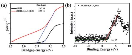
Fig. 6 (a) Tauc plot of OLHP and OLHP/S,N-GQD20 (b) valance band XPS of OLHP/S,N-GQD20
