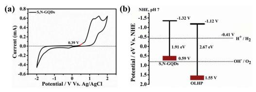
(a) Voltammogram of S,N-GQDs, (b) band energy diagram of S,N-GQDs and OLHP.
