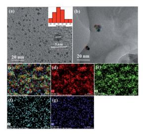
Fig. 2 (a) TEM images of S,N-GQDs (inset: particle size distribution and HRTEM of S,N-GQDs); (b) TEM image of OLHP/S,N-GQD20 and (c-g) the SEM elemental mapping of OLHP/S,N-GQD20.
