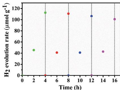
Fig. 9 Stability cycle of H<sub>2</sub> evolution of OLHP/S,N-GQD20.
