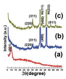
Fig. 2 XRD patterns data of (a) the synthesized GO powder, and (b) the Fe<sub>3</sub>O<sub>4</sub>/Ni foam and(c) Fe<sub>3</sub>O<sub>4</sub>@ reduced graphene oxide composite/Ni
