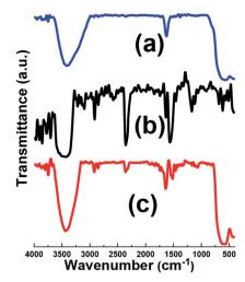
Fig. 3 IR spectra of (a) pristine Fe<sub>3</sub>O<sub>4</sub>, (b) GO and (c) Fe<sub>3</sub>O<sub>4</sub>@p-rGO composite
