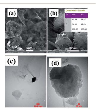
Fig. 5 (a and b) FE-SEM images, EDS data (inset in Fig. 4b), and (c and d) TEM images of the prepared graphene oxide.
