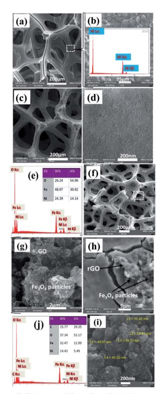
Fig. 6 FE-SEM images and EDS data of (a and b) blank Ni foam, and the fabricated (c–e) pristine  $Fe_3O_4$ @Ni foam and (f–j)  $Fe_3O_4$ /p-rGO@Ni foam.
