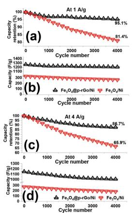
Fig. 12 (a and c) Capacity loss and (b and d) capacitance values and for the fabricated Fe $_3$ O $_4$ /NF and Fe $_3$ O $_4$ @p-rGO/NF electrodes within 4000 cycling at the discharge loads of 1 A g $^{-1}$  and 4 A g $^{-1}$ .
