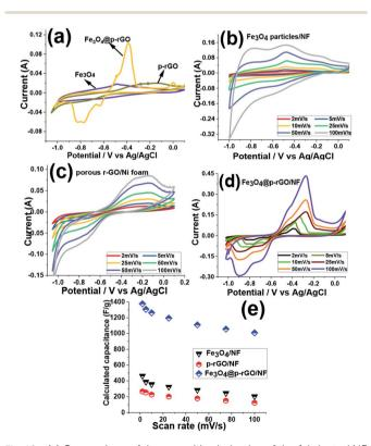
Fig. 10 (a) Comparison of the capacitive behavior of the fabricated NF electrodes at the scan rate of 5 mV s $^{-1}$ , (b-d) CVs of Fe $_3$ O $_4$ /NF, rGO/NF and Fe $_3$ O $_4$ @p $_7$ GO/NF at the scan rates of 2 $_7$ 100 mV s $^{-1}$ , (e) the calculated capacitances values vs. scan rate for the fabricated electrodes.
