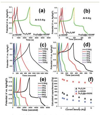
Fig. 11 (a and b) GCD profiles for the deposited active materials onto NF current collector at the current loads of 0.5 A g $^{-1}$  and 6 A g $^{-1}$  and the GCD profiles of (c) Fe $_3$ O $_4$ /NF, (d) rGO/NF and (e) Fe $_3$ O $_4$ @rGO/NF electrodes at various current loads within the range of 0.5 $^{-1}$ 0A g $^{-1}$  and (f) calculated specific capacitance values against current density for all electrodes.
