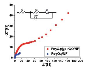
Fig. 13 The Nyquist plots for  $Fe_3O_4/NF$  and  $Fe_3O_4$ @p-rGO/NF electrodes. The inset shows the corresponding equivalent circuit pattern.
