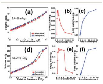
Fig. 9 BET and BJH pore size distribution curves of (a–c) pristine  $Fe_3O_4$  NPs and (d–f)  $Fe_3O_4$ @p-rGO composite.
