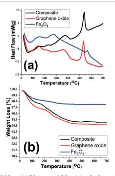
Fig. 8 (a) DSC and (b) TG curves of GO, pristine  $Fe_3O_4$  and  $Fe_3O_4$ @p-rGO composite.
