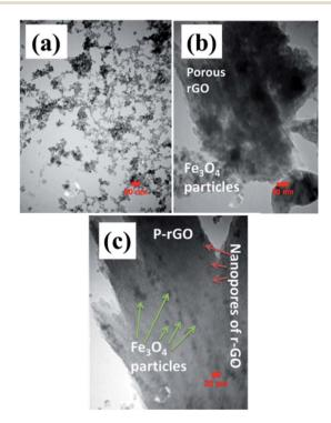
Fig. 7 TEM images of the synthesized (a) pristine  $Fe_3O_4$  and (b and c)  $Fe_3O_4/p\text{-r}GO.$
