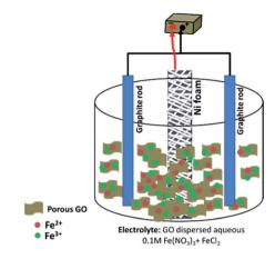
Fig. 1 Schematic view of the electrochemical set-up
