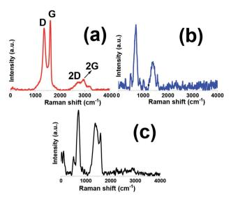
Fig. 4 Raman spectra of (a) GO, (b) pristine  $Fe_3O_4$  and (b)  $Fe_3O_4$ @p-rGO composite.
