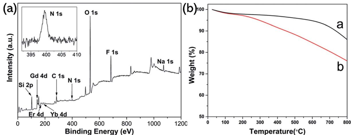
Fig. 3 (a) Survey XPS of UCNP@SiO<sub>2</sub>-SP. (b) TGA curve a of UCNPs@SiO<sub>2</sub> and curve b of UCNPs@SiO<sub>2</sub>-SP.
