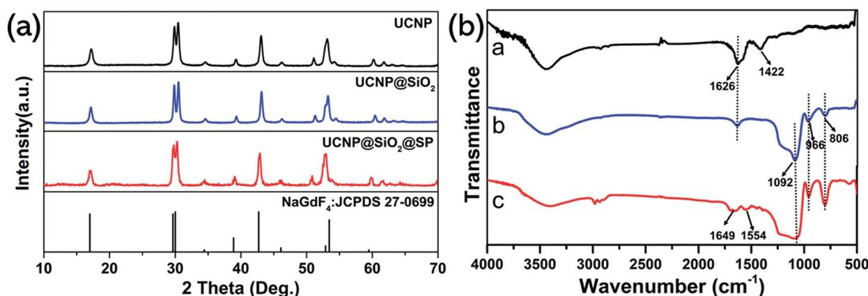
Fig. 2 (a) XRD patterns of UCNP, UCNP@SiO<sub>2</sub> and UCNP@SiO<sub>2</sub>-SP samples. The standard card of NaGdF<sub>4</sub> (JCPDS no. 27-0699) was given as a reference. (b) FTIR spectra of UCNP (curve a), UCNP@SiO<sub>2</sub> (curve b) and UCNP@SiO<sub>2</sub>-SP (curve c).
