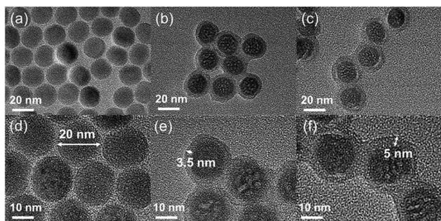
Fig. 1 TEM images of UCNP (a), UCNP@SiO<sub>2</sub> (b) and UCNP@SiO<sub>2</sub>-SP (c); HRTEM images of UCNP (d), UCNP@SiO<sub>2</sub> (e) and UCNP@SiO<sub>2</sub>-SP (f).
