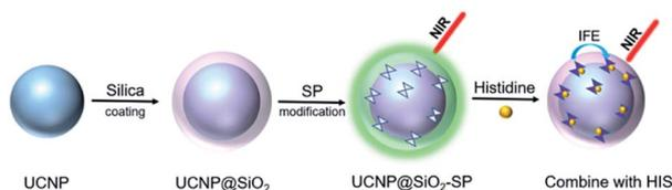
**Scheme 1** Schematic illustration of the preparation procedure of UCNPs@SiO<sub>2</sub>-SP nanosensor and detection process for His.
