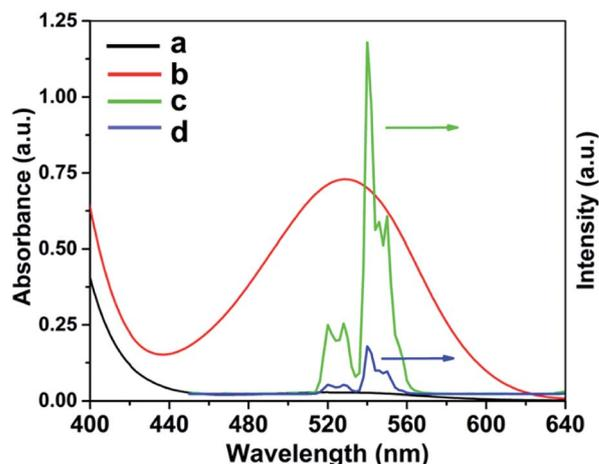
Fig. 7 UV-vis absorption spectrum of SP (curve a) and SP-His (curve b). Emission spectrum of UCNP@SiO<sub>2</sub>-SP (curve c) and UCNP@SiO<sub>2</sub>-SP with His under a 980 nm laser.
