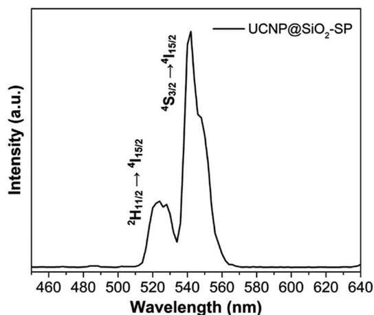
Fig. 4 The upconversion emission spectra of UCNP@SiO<sub>2</sub>-SP with a 980 nm laser.
