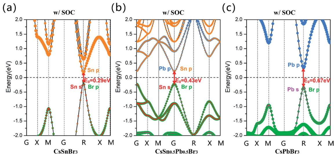
Fig. 2 Calculated projected band structures of (a) CsSnBr<sub>3</sub>, (b) CsSn<sub>0.5</sub>Pb<sub>0.5</sub>Br<sub>3</sub>, and (c) CsPbBr<sub>3</sub> obtained by the GGA + SOC method. The Fermi level was set at 0 eV and is denoted as a black dashed line.
