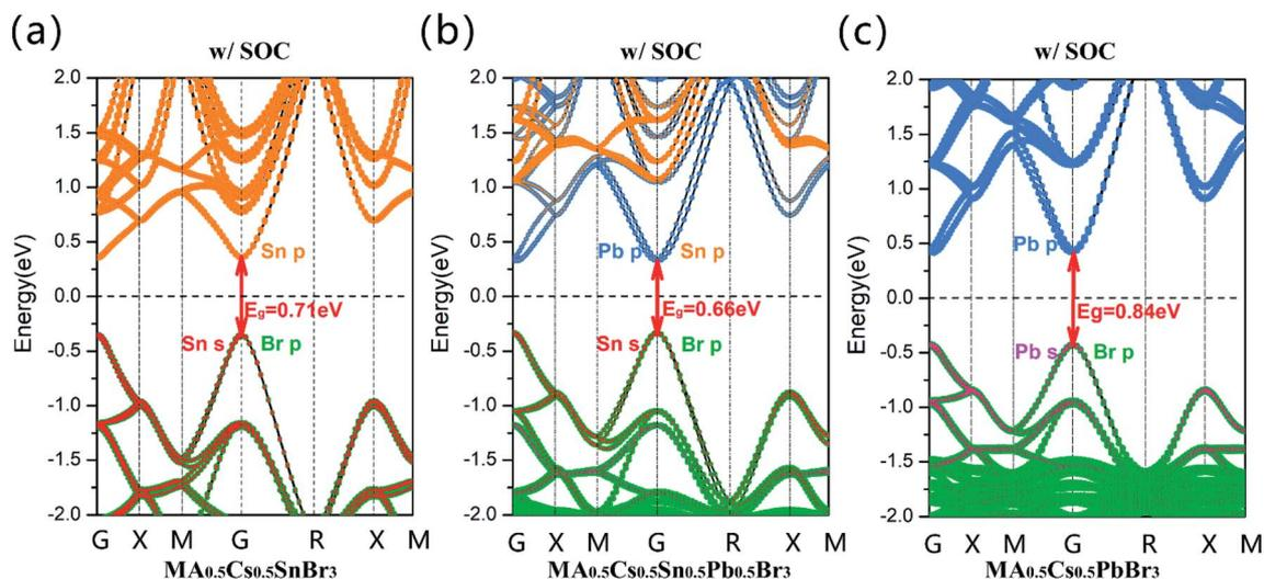
Fig. 3 Calculated projected band structures of (a) MA<sub>0.5</sub>Cs<sub>0.5</sub>SnBr<sub>3</sub>, (b) MA<sub>0.5</sub>Cs<sub>0.5</sub>Sn<sub>0.5</sub>Pb<sub>0.5</sub>Br<sub>3</sub>, and (c) MA<sub>0.5</sub>Cs<sub>0.5</sub>PbBr<sub>3</sub> obtained by the GGA + SOC method. The Fermi level was set at 0 eV and is denoted as a black dashed line.
