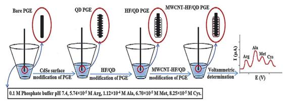
Fig. 3 Schematic of preparation of different modified electrodes with CdSe QD modified/MWCNT in 4 steps. Reprinted with permission from ref. 160 Copyright (2017) Elsevier.
