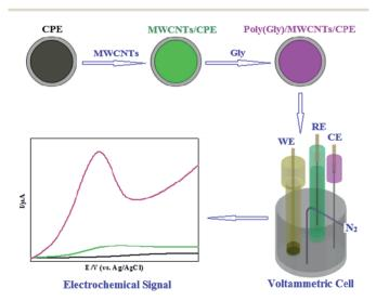
Fig. 4 Schematic illustration of glycine polymer and MWCNTs/CPE fabrication. Reprinted with permission from ref. 162 Copyright (2018) Electrochemical Science Group, University of Belgrade.
