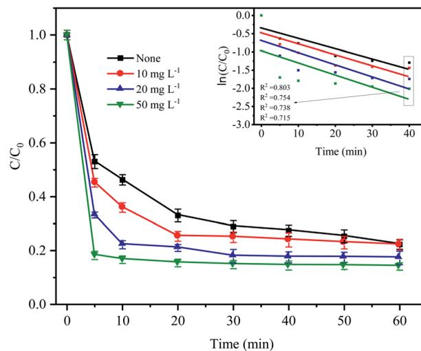
Fig. 8 Effect of humic acid on CTC degradation in Fe<sup>0</sup>-AC/PDS system. Experimental conditions: [CTC] = 50 mg L<sup>-1</sup>, [PDS] = 2 g L<sup>-1</sup>, [Fe<sup>0</sup>] = 0.4 g L<sup>-1</sup>, [AC] = 0.2 g L<sup>-1</sup>, and pH = 5.
