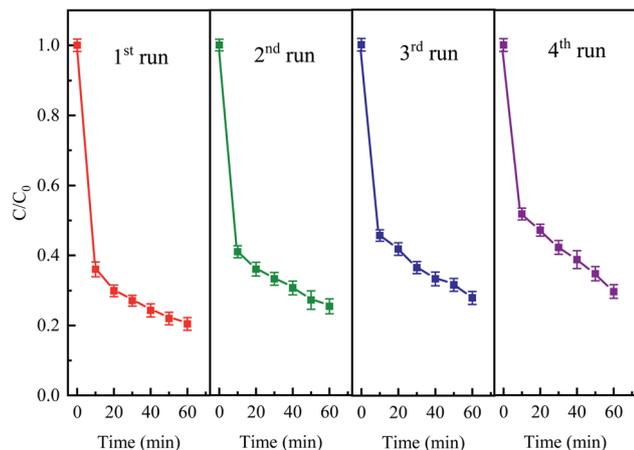
Fig. 11 The degradation of CTC in Fe<sup>0</sup>-AC/PDS system within the successive four cycles. Experimental conditions: [CTC] = 50 mg L<sup>-1</sup>, [PDS] = 2 g L<sup>-1</sup>, [Fe<sup>0</sup>] = 0.4 g L<sup>-1</sup>, [AC] = 0.2 g L<sup>-1</sup>, and pH = 5.
