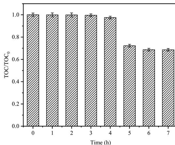
Fig. 9 TOC removals on CTC degradation by in Fe<sup>0</sup>-AC/PDS system. TOC<sub>0</sub> is the initial organic carbon value and TOC is the organic carbon value at t (h). Experimental conditions: [CTC] = 50 mg L<sup>-1</sup>, [PDS] = 2 g L<sup>-1</sup>, [Fe<sup>0</sup>] = 0.4 g L<sup>-1</sup>, [AC] = 0.2 g L<sup>-1</sup>, initial pH = 5, and the final pH = 3.12.
