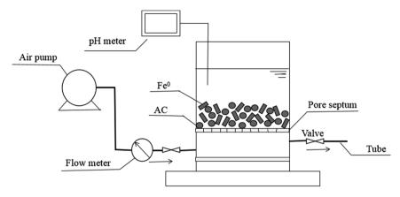
Fig. 1 The schematic diagram of the reactor for continuous experiment
