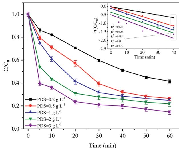
Fig. 4 Effect of PDS dose on CTC degradation in  $\text{Fe}^0$ -AC/PDS system. Experimental conditions: [CTC] =  $50 \text{ mg L}^{-1}$ , [ $\text{Fe}^0$ ] =  $0.4 \text{ g L}^{-1}$ , [AC] =  $0.2 \text{ g L}^{-1}$  and pH = 5.
