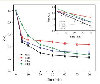
Fig. 10 Effect of radical scavengers on CTC degradation in Fe $^0$ -AC/PDS system. Experimental conditions: [CTC] = 50 mg L $^{-1}$ , [PDS] = 2 g L $^{-1}$ , [Fe $^0$ ] = 0.4 g L $^{-1}$ , [AC] = 0.2 g L $^{-1}$ , pH = 5, and [EtOH] = [TBA] = [PBQ] = 50 mM.
