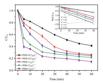
Fig. 4 Effect of PDS dose on CTC degradation in Fe $^0$ -AC/PDS system. Experimental conditions: [CTC] = 50 mg L $^{-1}$ , [Fe $^0$ ] = 0.4 g L $^{-1}$ , [AC] = 0.2 g L $^{-1}$  and pH = 5.
