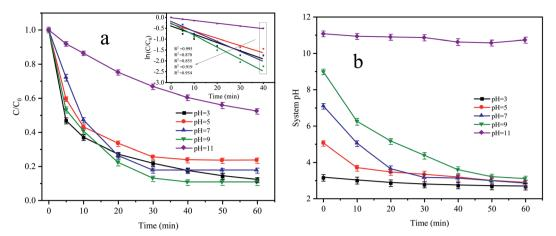
Fig. 5 (a) Effect of initial pH on CTC degradation in Fe $^0$ -AC/PDS system and (b) variation curve of system pH during the reaction. Experimental conditions: [CTC] = 50 mg L $^{-1}$ , [PDS] = 2 g L $^{-1}$ , [Fe $^0$ ] = 0.4 g L $^{-1}$  and [AC] = 0.2 g L $^{-1}$ .
