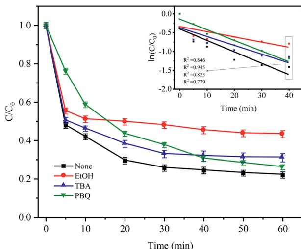
Fig. 10 Effect of radical scavengers on CTC degradation in  $\text{Fe}^0$ -AC/PDS system. Experimental conditions:  $[\text{CTC}] = 50 \text{ mg L}^{-1}$ ,  $[\text{PDS}] = 2 \text{ g L}^{-1}$ ,  $[\text{Fe}^0] = 0.4 \text{ g L}^{-1}$ ,  $[\text{AC}] = 0.2 \text{ g L}^{-1}$ ,  $\text{pH} = 5$ , and  $[\text{EtOH}] = [\text{TBA}] = [\text{PBQ}] = 50 \text{ mM}$ .
