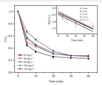
Fig. 6 Effect of the initial CTC concentration on CTC degradation in  $Fe^0$ -AC/PDS system. Experimental conditions: [PDS] = 2 g L<sup>-1</sup>, [Fe<sup>0</sup>] = 0.4 g L<sup>-1</sup>, [AC] = 0.2 g L<sup>-1</sup>, and pH = 5.
