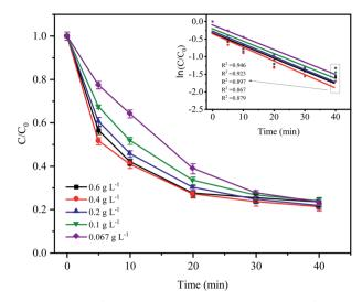
Fig. 3 Effect of Fe<sup>0</sup> dose on the degradation of CTC in Fe<sup>0</sup>–AC/PDS system. Experimental conditions: [CTC] = 50 mg L<sup>-1</sup>, [PDS] = 2 g L<sup>-1</sup>, [AC] = 0.2 g L<sup>-1</sup> and pH = 5.
