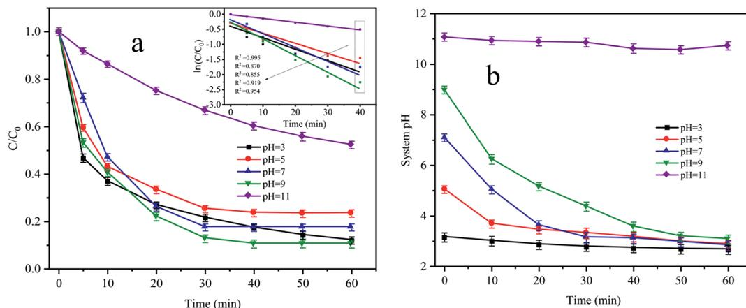
Fig. 5 (a) Effect of initial pH on CTC degradation in  $\text{Fe}^0\text{-AC/PDS}$  system and (b) variation curve of system pH during the reaction. Experimental conditions:  $[\text{CTC}] = 50 \text{ mg L}^{-1}$ ,  $[\text{PDS}] = 2 \text{ g L}^{-1}$ ,  $[\text{Fe}^0] = 0.4 \text{ g L}^{-1}$  and  $[\text{AC}] = 0.2 \text{ g L}^{-1}$ .
