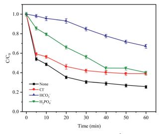
Fig. 7 Effects of anions on CTC degradation in Fe $^0$ -AC/PDS system. Experimental conditions: [CTC] = 50 mg L $^{-1}$ , [PDS] = 2 g L $^{-1}$ , [Fe $^0$ ] = 0.4 g L $^{-1}$ , [AC] = 0.2 g L $^{-1}$ , pH = 5 and [Cl $^-$ ] = [HCO $_3$  $^-$ ] = [H $_2$ PO $_4$  $^-$ ] = 100 mM.
