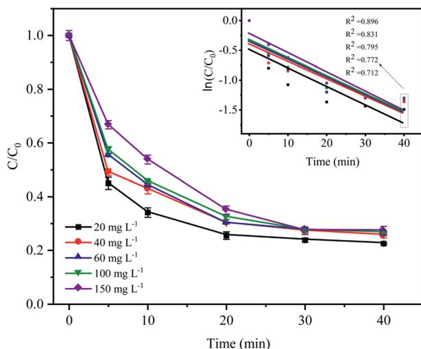
Fig. 6 Effect of the initial CTC concentration on CTC degradation in  $\text{Fe}^0\text{-AC/PDS}$  system. Experimental conditions:  $[\text{PDS}] = 2 \text{ g L}^{-1}$ ,  $[\text{Fe}^0] = 0.4 \text{ g L}^{-1}$ ,  $[\text{AC}] = 0.2 \text{ g L}^{-1}$ , and  $\text{pH} = 5$ .
