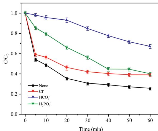
Fig. 7 Effects of anions on CTC degradation in  $\text{Fe}^0\text{-AC/PDS}$  system. Experimental conditions:  $[\text{CTC}] = 50 \text{ mg L}^{-1}$ ,  $[\text{PDS}] = 2 \text{ g L}^{-1}$ ,  $[\text{Fe}^0] = 0.4 \text{ g L}^{-1}$ ,  $[\text{AC}] = 0.2 \text{ g L}^{-1}$ ,  $\text{pH} = 5$  and  $[\text{Cl}^-] = [\text{HCO}_3^-] = [\text{H}_2\text{PO}_4^-] = 100 \text{ mM}$ .
