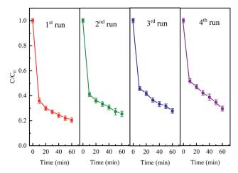
Fig. 11 The degradation of CTC in Fe $^0$ -AC/PDS system within the successive four cycles. Experimental conditions: [CTC] = 50 mg L $^{-1}$ , [PDS] = 2 g L $^{-1}$ , [Fe $^0$ ] = 0.4 g L $^{-1}$ , [AC] = 0.2 g L $^{-1}$ , and pH = 5.
