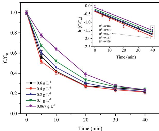
Fig. 3 Effect of  $\text{Fe}^0$  dose on the degradation of CTC in  $\text{Fe}^0$ -AC/PDS system. Experimental conditions: [CTC] =  $50 \text{ mg L}^{-1}$ , [PDS] =  $2 \text{ g L}^{-1}$ , [AC] =  $0.2 \text{ g L}^{-1}$  and pH = 5.
