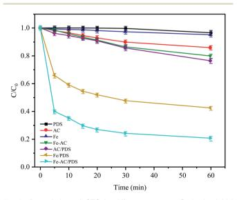
Fig. 2 Degradation of CTC in different systems.  $C_0$  is the initial concentration of CTC and C is the concentration at time t (min). Experimental conditions: [CTC] = 50 mg L<sup>-1</sup>, [PDS] = 2 g L<sup>-1</sup>, [Fe<sup>0</sup>] = 0.4 g L<sup>-1</sup>, [AC] = 0.2 g L<sup>-1</sup> and pH = 5.
