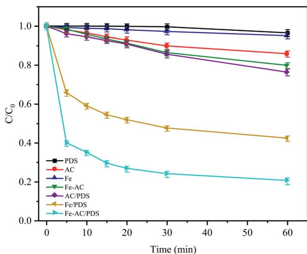
Fig. 2 Degradation of CTC in different systems.  $C_0$  is the initial concentration of CTC and  $C$  is the concentration at time  $t$  (min). Experimental conditions:  $[\text{CTC}] = 50 \text{ mg L}^{-1}$ ,  $[\text{PDS}] = 2 \text{ g L}^{-1}$ ,  $[\text{Fe}^0] = 0.4 \text{ g L}^{-1}$ ,  $[\text{AC}] = 0.2 \text{ g L}^{-1}$  and  $\text{pH} = 5$ .
