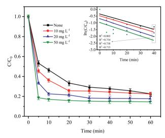
Fig. 8 Effect of humic acid on CTC degradation in Fe $^0$ -AC/PDS system. Experimental conditions: [CTC] = 50 mg L $^{-1}$ , [PDS] = 2 g L $^{-1}$ , [Fe $^0$ ] = 0.4 g L $^{-1}$ , [AC] = 0.2 g L $^{-1}$ , and pH = 5.
