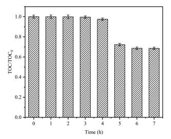
Fig. 9 TOC removals on CTC degradation by in Fe $^0$ -AC/PDS system. TOC $_0$  is the initial organic carbon value and TOC is the organic carbon value at t (h). Experimental conditions: [CTC] = 50 mg L $^{-1}$ , [PDS] = 2 g L $^{-1}$ , [Fe $^0$ ] = 0.4 g L $^{-1}$ , [AC] = 0.2 g L $^{-1}$ , initial pH = 5, and the final pH = 3.12
