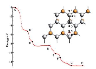
Fig. 5 An energy curve indicates that the Li atom starts from far away, along the gradient direction of potential energy to  $CF_x$  surface, and then reaches the optimal structure of  $C_{32}F_{16}Li$  system. And several important nodes A–H are marked.
