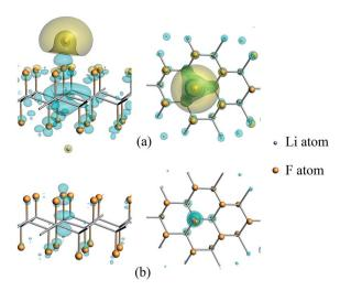
**Fig. 4** Charge density difference of Li atom adsorbed on  $CF_x$  surface, with the iso-surface level of 0.0015. The space enclosed by the blue and yellow iso-surfaces are the electron gaining and losing regions, respectively. (a) and (b) show the cases when the Li–F distance are 1.71 and 3.00 Å, respectively. Left and right are side view and top view of the system.
